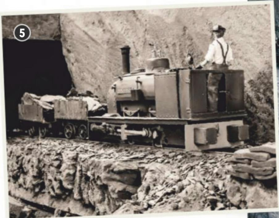
locomotives to run on tracks narrower than 4ft 8½in. The Festiniog Railway became the first steam-worked narrow gauge railway.
