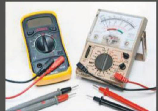
Resistance, voltage flow and many other tests can be carried out, along with testing batteries for charge. At the simplest level, however, the continuity test function is the most useful, helping us to identify any breaks in a circuit using a pair of contact probes. Full instructions are supplied with each tool and plenty of tutorials can be found online.
