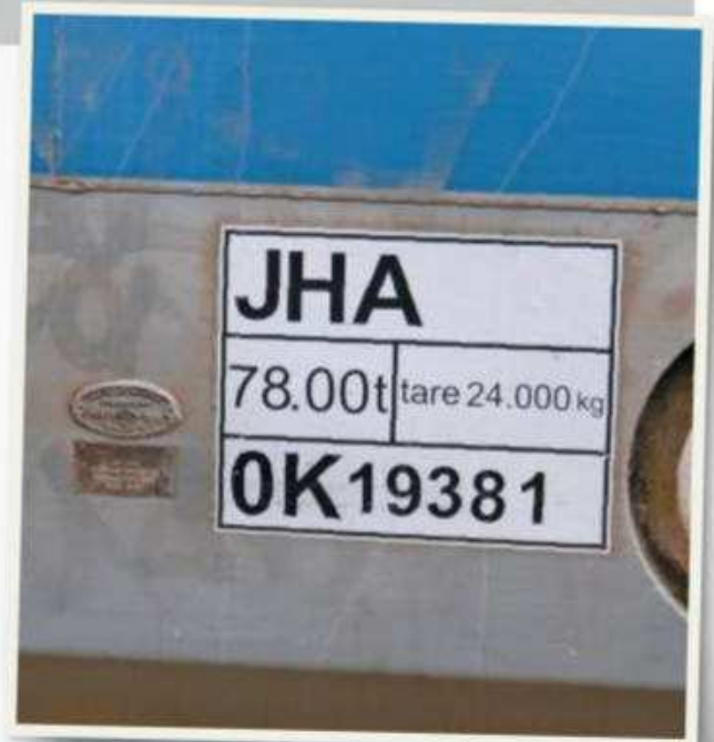
Above: With a payload capacity of 78t, the JHAs have allowed Yeoman to shift ever greater tonnages of stone from the Mendip quarries. GEORGE DENT
