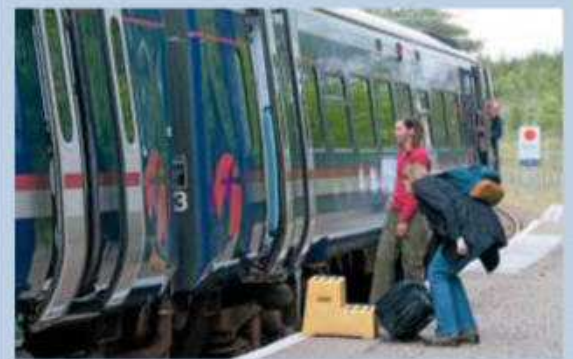
Not all platforms are the same height. Those at Forsinard, on the Far North line, are so low that plastic steps are provided to bridge the gap. VINCENT LOWE/ALAMY
