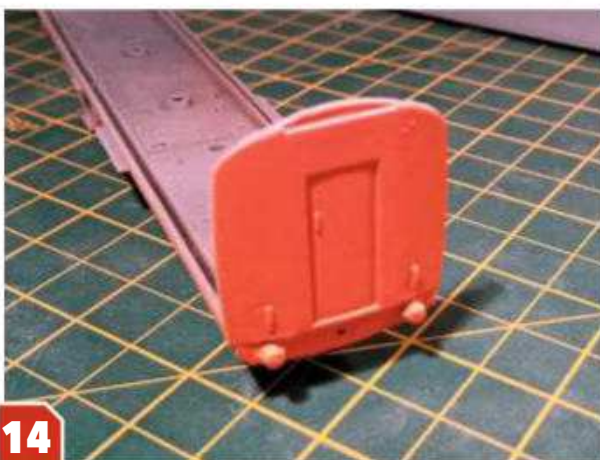
14 The buffers and moulded coupling hooks were also carved away. After priming and under-coating in white (see panel, page 41), Plastikote Fluorescent Red was applied with an aerosol.
