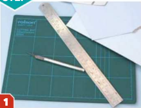
1 Cut out the platform shape using a cutting mat, a steel rule and sharp craft knife. Use a fresh blade and made the cuts slowly. Use fine sandpaper to smooth the edges of the cut cardboard.
