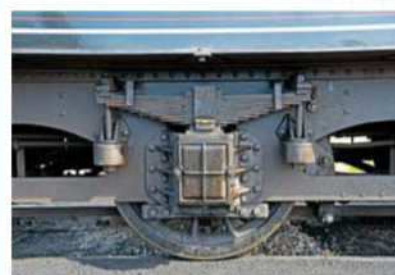
The first 50 'Black Fives' had tenders with plain axlebox covers. This cross pattern became the standard, except for machines fitted with roller bearings.
