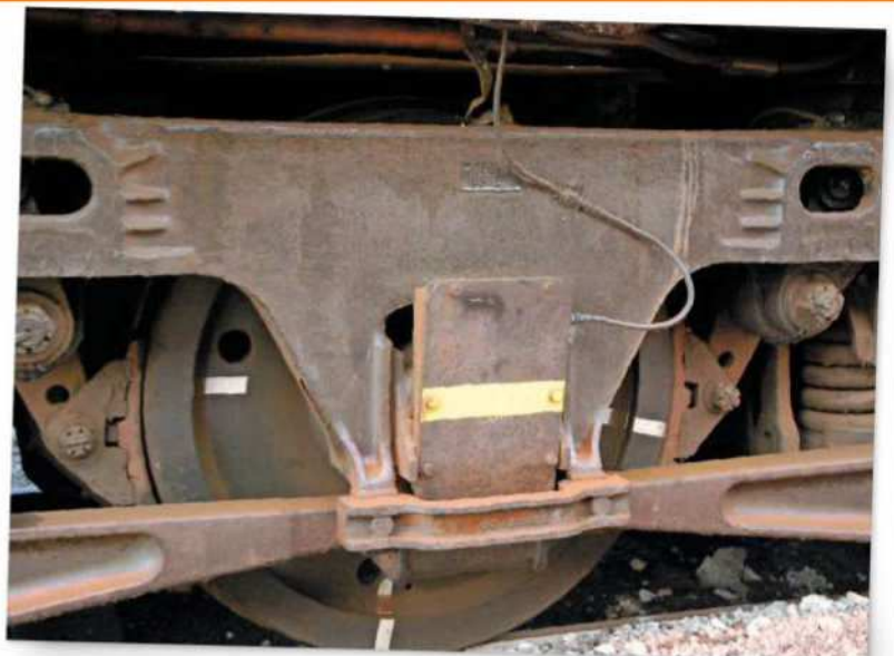
Above: The flat, rectangular cover of the speedometer drive, as fitted to the No. 2 end bogie of preserved 'Royal' Class 47 47798, on February 2011. GEORGE DENT
