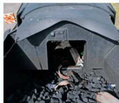
The coal space, complete with weather protection.
