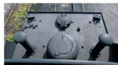
Welded tenders have these extended 'mush-room' vents. Part-welded tenders have squarer vents closer to the coal space.
