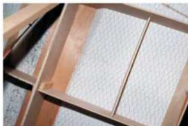
A view of Graham's innovative 'T' beam baseboards. The 'T' is formed from 120mm and 100mm wide strips of 9mm plywood, glued and screwed together. The scenery supports a cantilever off the 'T'.
