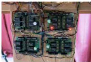
Left: This piece of electronic wizardry switches power from Track 1 to Track 2 to enable the banking locomotive to drop off an uphill train and reverse down the bank. Prototypical operation without DCC!
