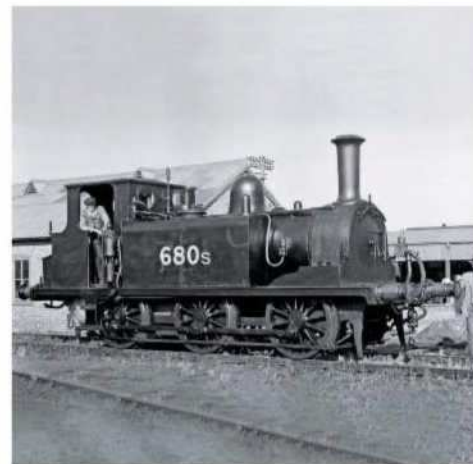
Waddon , as Departmental No. DS680, at Lancing Carriage Works in August 1933. It had been fitted with a Wainwright boiler in 1910, but retained its 'A1' smokebox. It later gained an 'A1X' boiler but the original smokebox remained, and it's in this condition that it has been preserved... in Canada! O.J. MORRIS/RAIL ARCHIVE STEPHENSON
