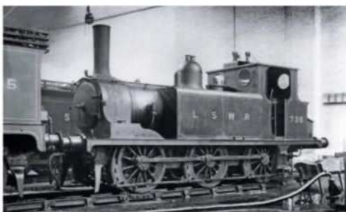
LSWR 'Terrier' No. 735, formerly LBSCR Clapham , at an unknown location. Its Drummond boiler, with safety valves atop the dome, stovepipe chimney, and pulley and wire control for working motor trains on the Lee-on-Solent Light Railway, is clearly visible. BERNARD WHICHER/RAIL ARCHIVE STEPHENSON
