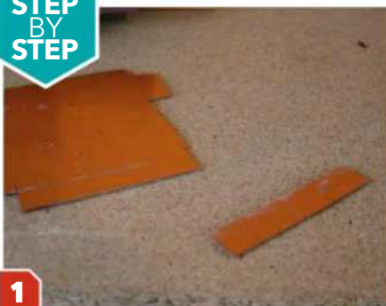
1 Cut a strip from the copper-clad glass fibre sheet. A razor saw or junior hacksaw works well, though be aware that the sheet's edges can be sharp.
