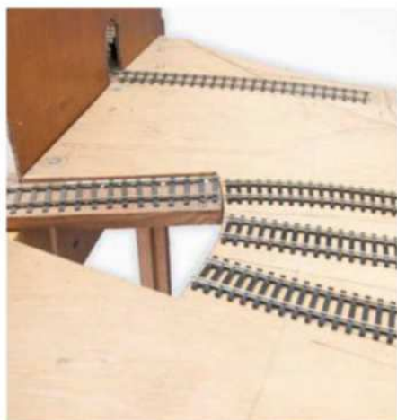
Sector plates can be made to almost any length. Smaller plates can handle locomotives only, replacing the need for points and a headshunt in a run-round loop.
