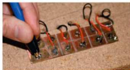
...while touching the probe against the red wire switches the solenoid back the other way.
