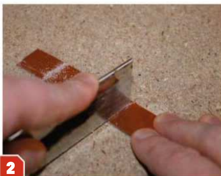
2 Use a sharp blade - a razor saw in this case - to score through the copper. Divide the strip into six.
