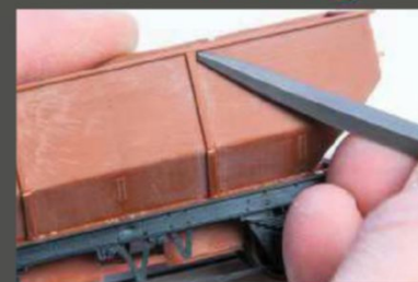
Riffler files can work into tight, awkward corners, making them great for fettling kit parts before or during assembly.
