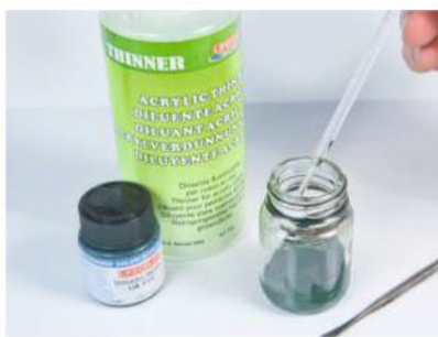
For best results, use the same brand of paints and thinners, combining both in a glass mixing jar before loading the airbrush. The paint needs to be about the same viscosity as milk.
