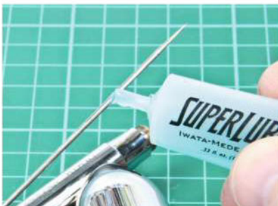
A drop of lubricant on the needle and trigger keeps the internal components working effectively.
