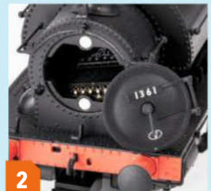
2 DCC socket inside smokebox.
