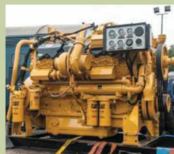
One of the compact 950hp CAT 12-cylinder diesel power units, as fitted within the Class 88s.
