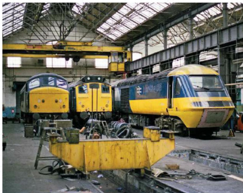
British Rail Engineering Ltd at Litchurch Lane, Derby, in full flow in 1983. The ex-Midland Railway works not only churned out dozens of four-wheel chassis for the 'Pacer' fleet but provided overhaul facilities to all manner of BR diesel classes, including Classes 45, 25 and 43.
