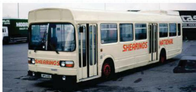
British Leyland's monocoque, modular, riveted National single-deck bus was first unveiled at the 1970 Commercial Motor Show. Production commenced in 1972, but a lack of orders forced BL to look for other markets. This Shearings Mk 1 was one of the 11.3m vehicles, identified by its second set of doors. Both have a flatter, less bulbous front end, as opposed to the Mk 2 versions, as seen on LEV 2.
