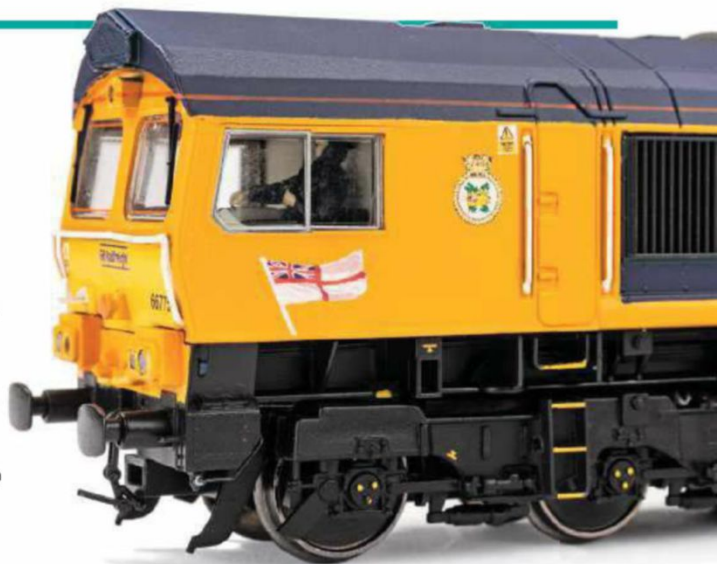
17 Finally, when thoroughly dry, give them a coat of water-based varnish, allow to dry then spray with standard RailMatch satin varnish.
