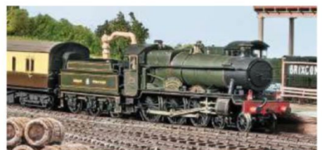
'Hall' 4-6-0 No. 4906 Bradfield Hall - Martin Finney kit with Ultrascaple wheels and Portescap RG4 motor and gearbox.
