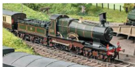
'City' 4-4-0 No. 3433 City of Bath in 1903 monogram livery - Martin Finney kit with Portescap RG4 motor and gears.
