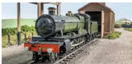
'Grange' 4-6-0 No. 6837 Fordhampton Grange - Malcolm Mitchell kit, Ultrascaple wheels and Portescap RG4 motor and gearbox.
