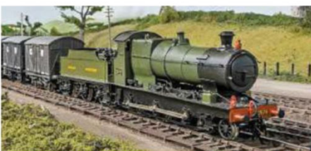
'Aberdare' 2-6-0 No. 2676 - Martin Finney kit with working inside crank shafts. Portescap RG4 motor and gearbox.
