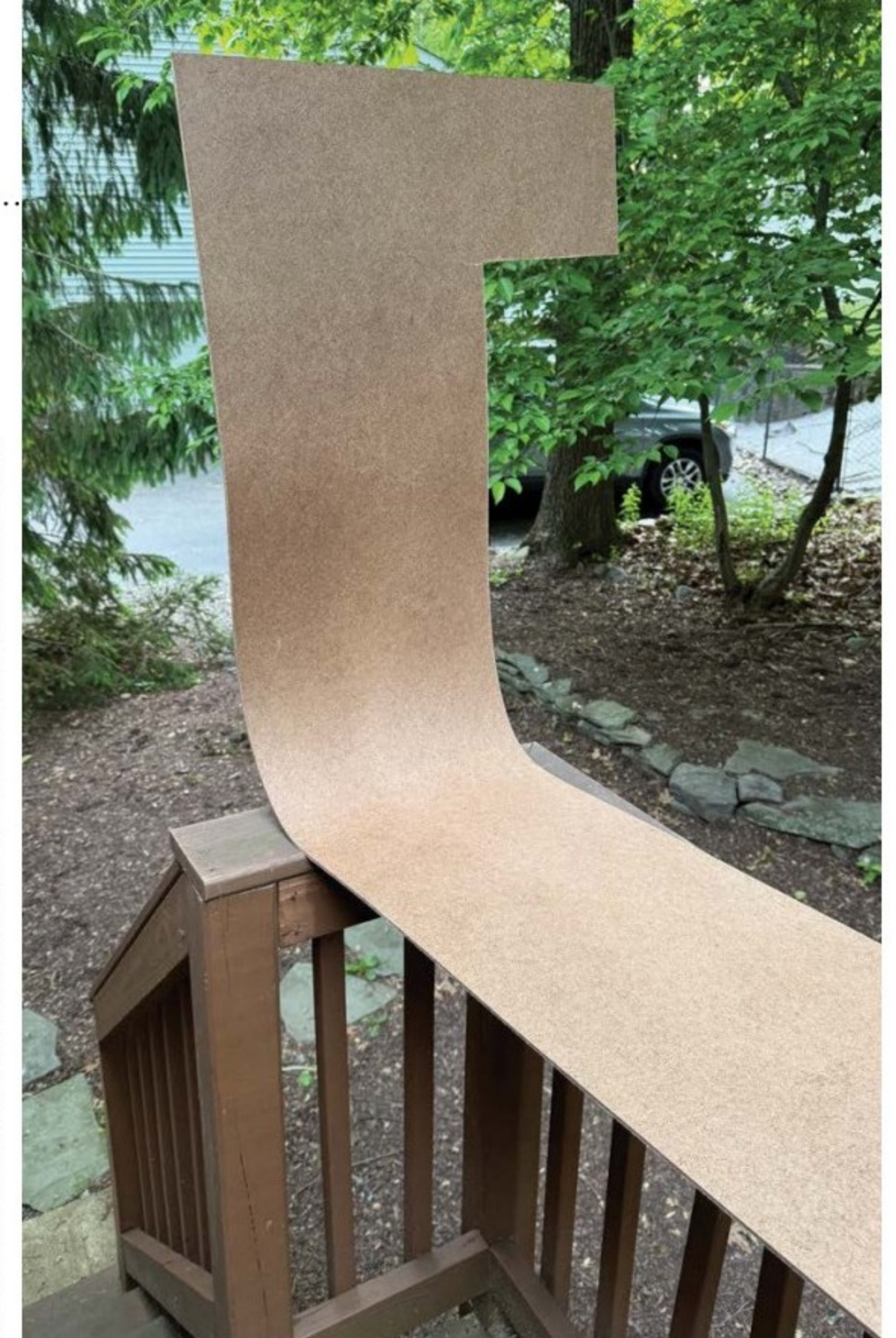
Model Railroader Consulting Editor Tony Koester needed a 12"-radius curve in his tempered hardboard backdrop. After spraying the panel with Windex window cleaner and ammonia, he weighted down the long end and clamped the short end to the balusters on his porch. The finished backdrop is shown above. As you can see, the tempered hardboard holds its shape nicely. Tony Koester photo
