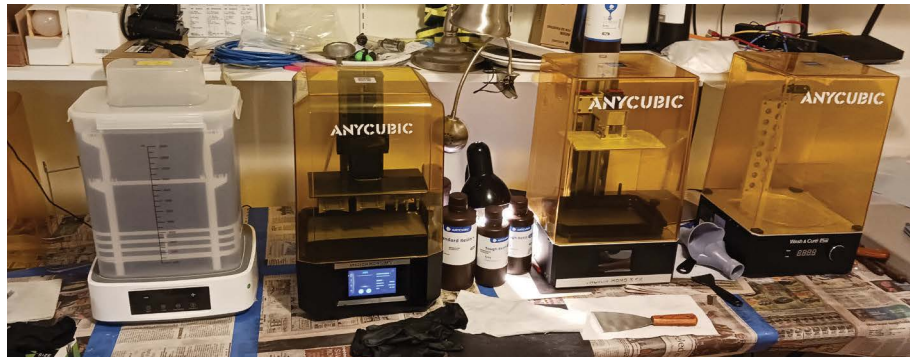
2 The M5s is the center left machine while the 6K is at the center right. These are flanked by a pair of Anycubic's wash and cure machines. On some projects Steve has kept both printers running every day for a month.
