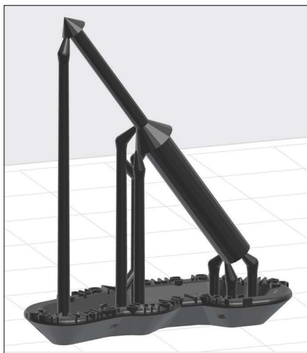
21 Supports were automatically added to this simple smoke vent by Preform after Steve oriented the part. Complex shapes are more likely to require reorientation or support editing to ensure proper printing.
