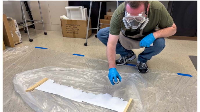
Cody applied 3M Super 77 adhesive to the back of the paper backdrops, using scrap boards to hold the ends flat and keep the paper section from moving.
