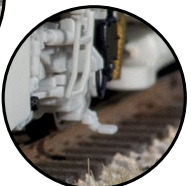
MNCR Lowered Position Lowered or raised third rail shoes
