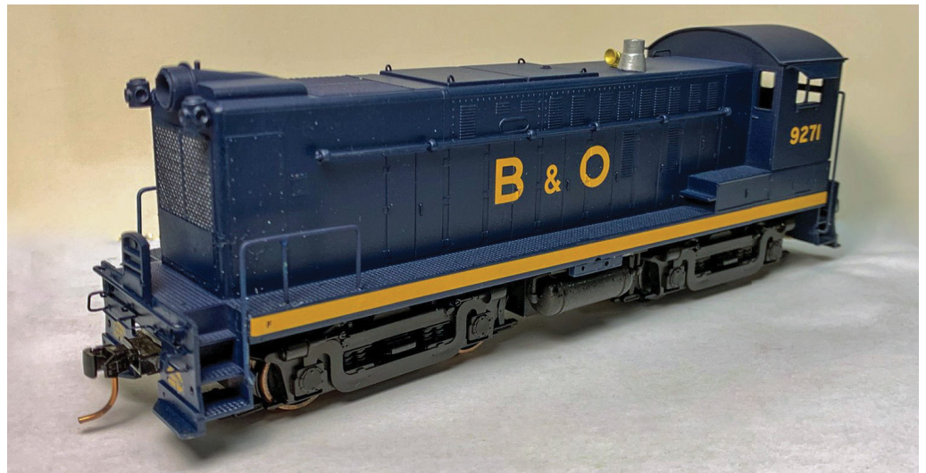
7 That new paint smell. Here's how the switcher looked after Brooks painted and decaled it. He brush-painted the exhaust stack aluminum.
