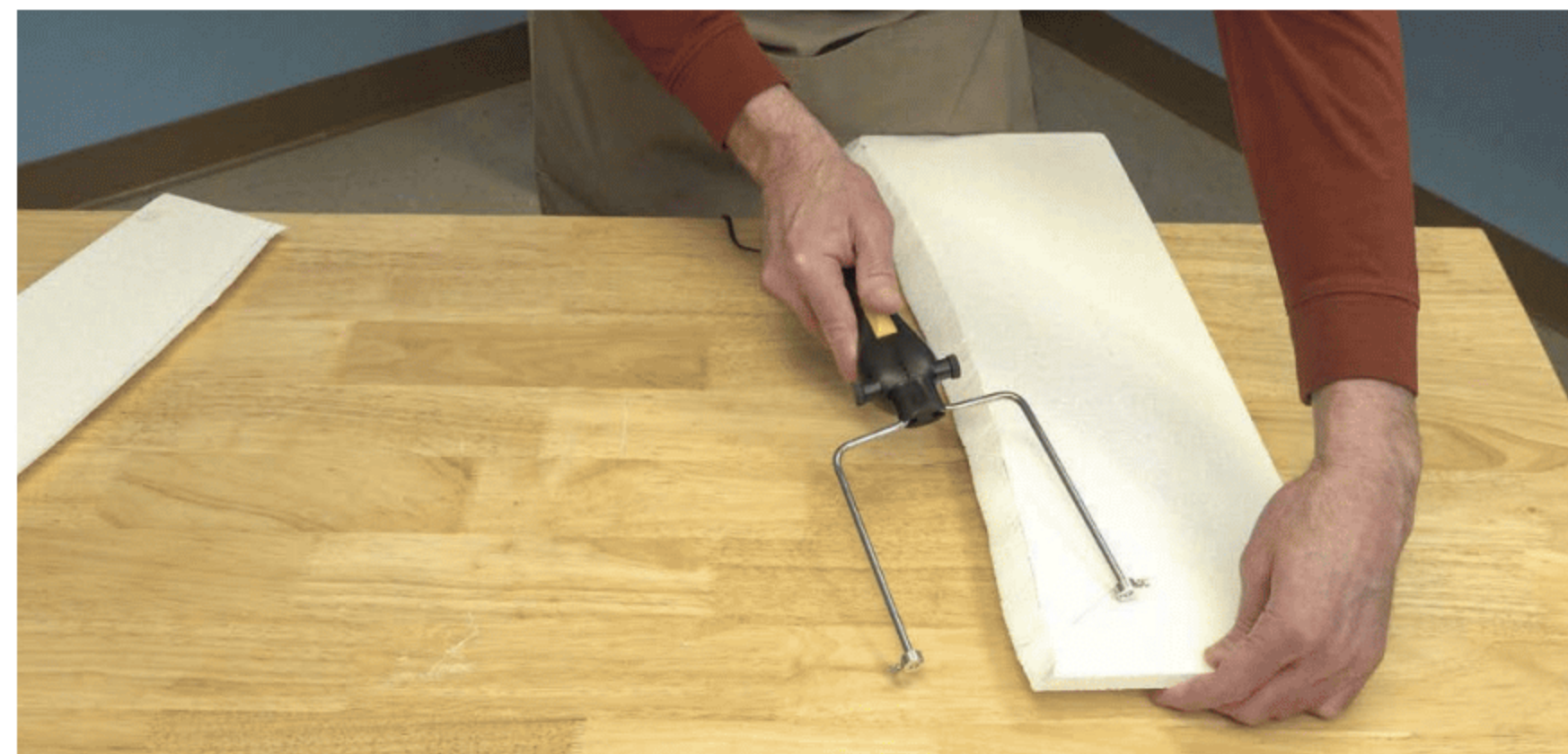
The foam is easy to cut and shape with assorted hobby knives, as well as with a hot wire foam cutting tool, as shown here.
