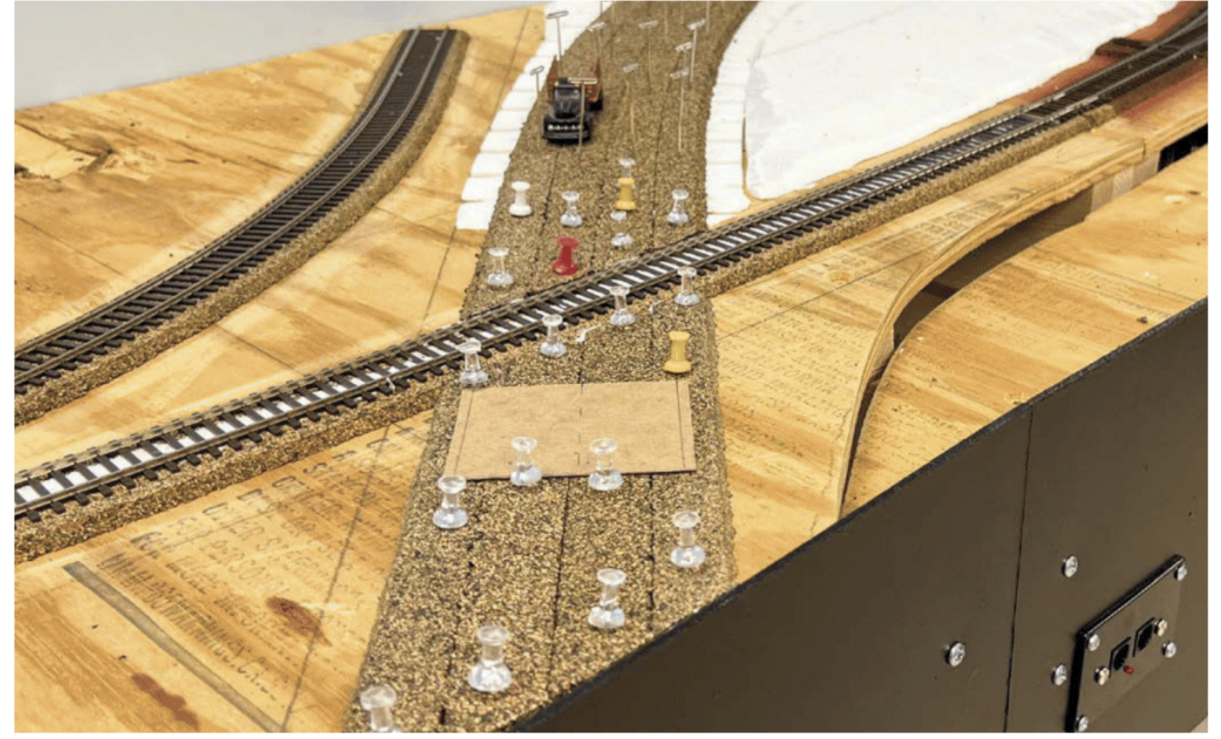
Pushpins held the cork strips to the plywood and foam surfaces until the caulk set, particularly through the curve and the approaches to the tracks.
