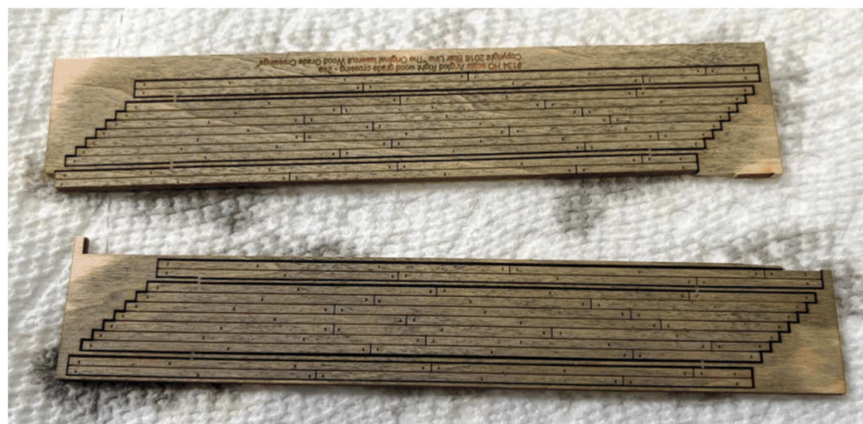
David used a laser-cut wood HO scale angled grade crossing kit from Blair Line, staining it with India ink and gluing it to the ties of the track with gel-type cyanoacrylate adhesive.
