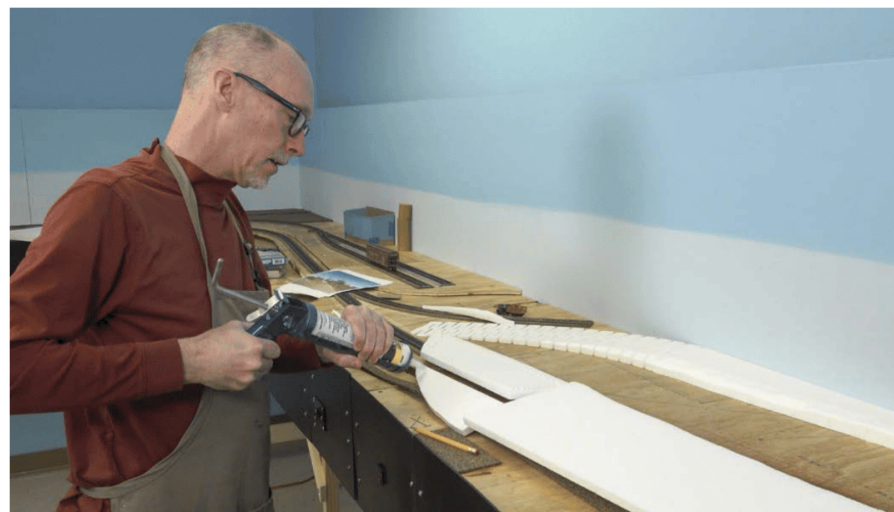
David glued the foam to the layout's plywood top using DAP acrylic latex caulk, letting the caulk cure overnight before continuing scenery construction.
