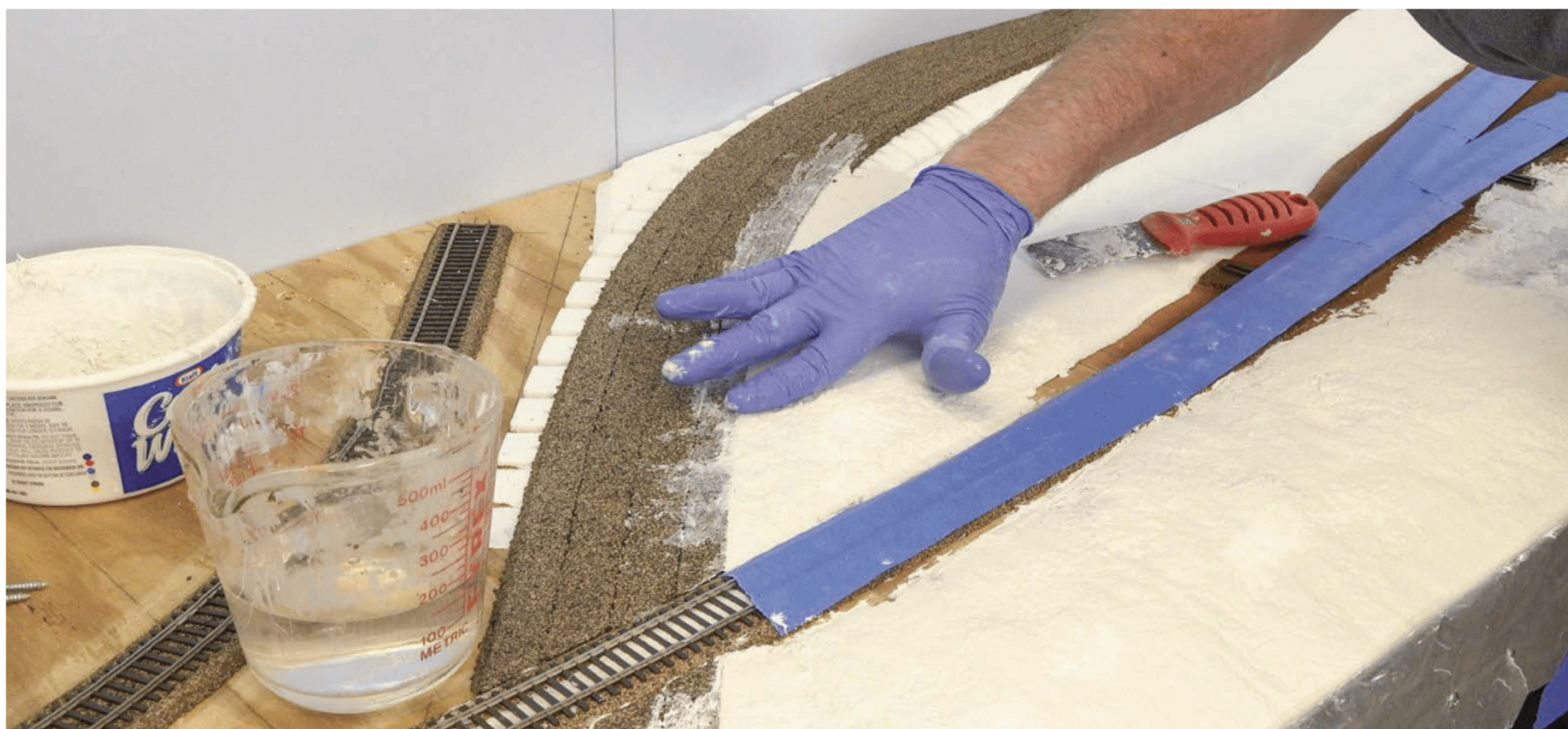
To smooth the surface of the Sculptamold, David dipped his fingertips in water and then ran them over the scenery, looking for lumps or rough spots.
