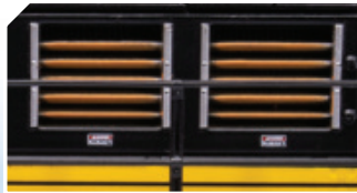
DYNAMIC BRAKE CAB (FIREMAN'S SIDE) High-capacity dynamic brake exhaust (2-port)
