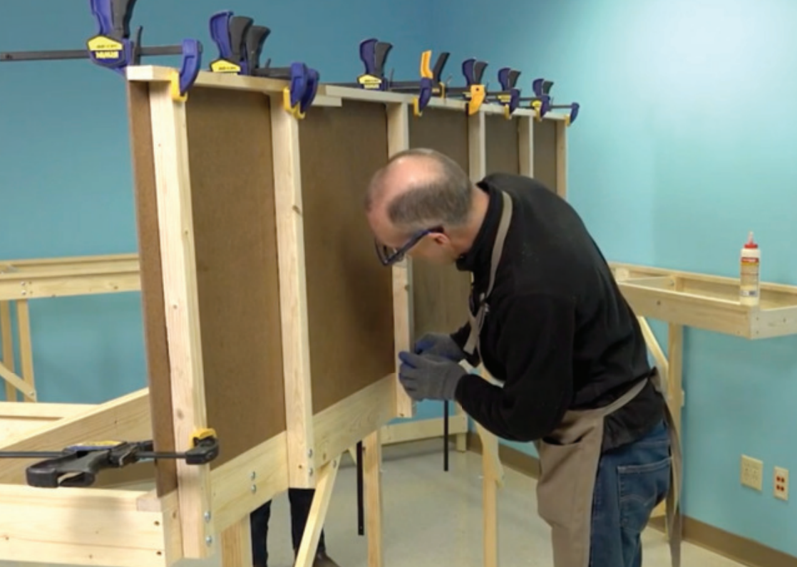
The backdrop is also removable and is made from a framework of 2 x 2 posts and a 1 x 2 top cap with \frac{3}{16} " hardboard glued to it. It bolts to the L-girder along the back of the layout.
