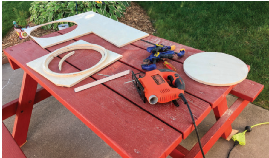
Dennis cut the round shapes for the pit wall from \frac{1}{2} " plywood using a jig saw. The messy sawing was done outdoors. A leaf blower made the clean up easy.
