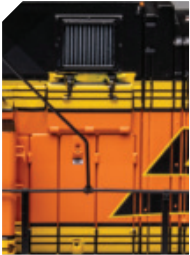
AUXILIARY CAB (FIREMAN'S SIDE) 3 short doors with latches on the #2 door and narrow auxiliary cab filter box door
