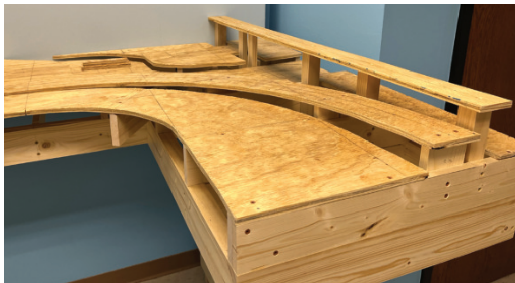
The Mukwonago end of the layout has the most elevation changes, including the CN main line, the interchange track, and the riverbed. All were accomplished using risers or by cutting 1" deep notches in the stringers. All screws are countersunk below the plywood's surface.
