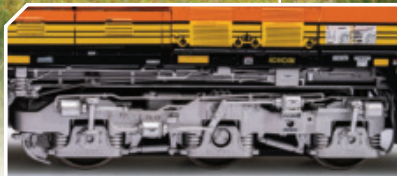
TRUCK DETAILS "C4" A-1-A trucks with idler center axle and weight management system
