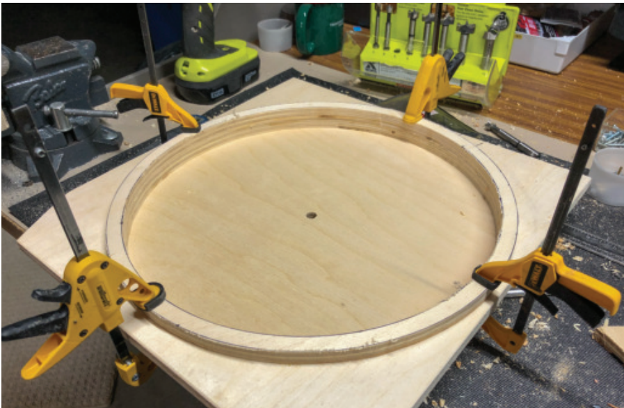
Next, Dennis used small bar clamps to hold the rough assembly of the pit wall together until the wood glue dried.
