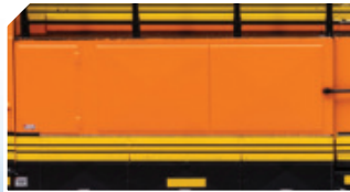
INVERTER CABINET (FIREMAN'S SIDE) With bolted and hinged access door, top two X panels same size, three lower X panels with 4 - 6 - 4 bolt pattern
