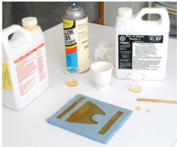
**8 Making multiples.** Howard used Synair Corp. products, purchased at a local art supply store, to cast the parts for the culvert. The company's mold release is in the aerosol can; its two-part resin is in the plastic jugs.
