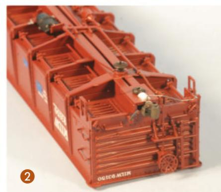
The ready-to-run InterMountain model I purchased is decorated as Milwaukee Road No. 93150 in its 1949 as-delivered appearance. However, when I examined the model more closely, I noticed the air reservoir for the AB brake system was missing. However, the brackets were there.
