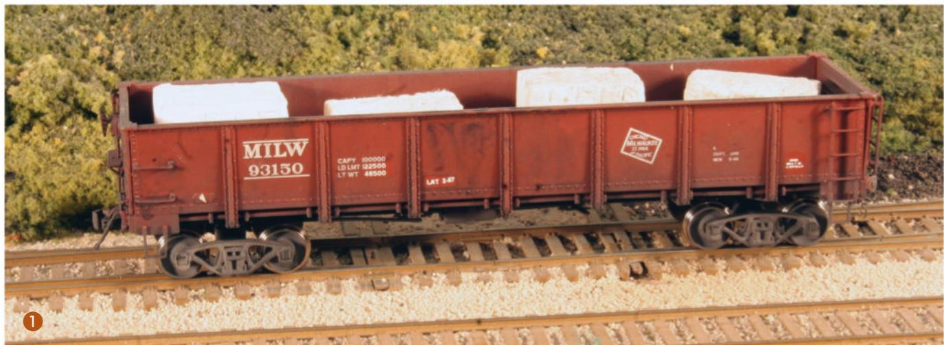
With the black wash satisfactorily applied, I removed the bits of masking tape from the sides of the car, exposing the light weight and load limit lettering. The numbers should look clean compared to the data that wasn't masked.
