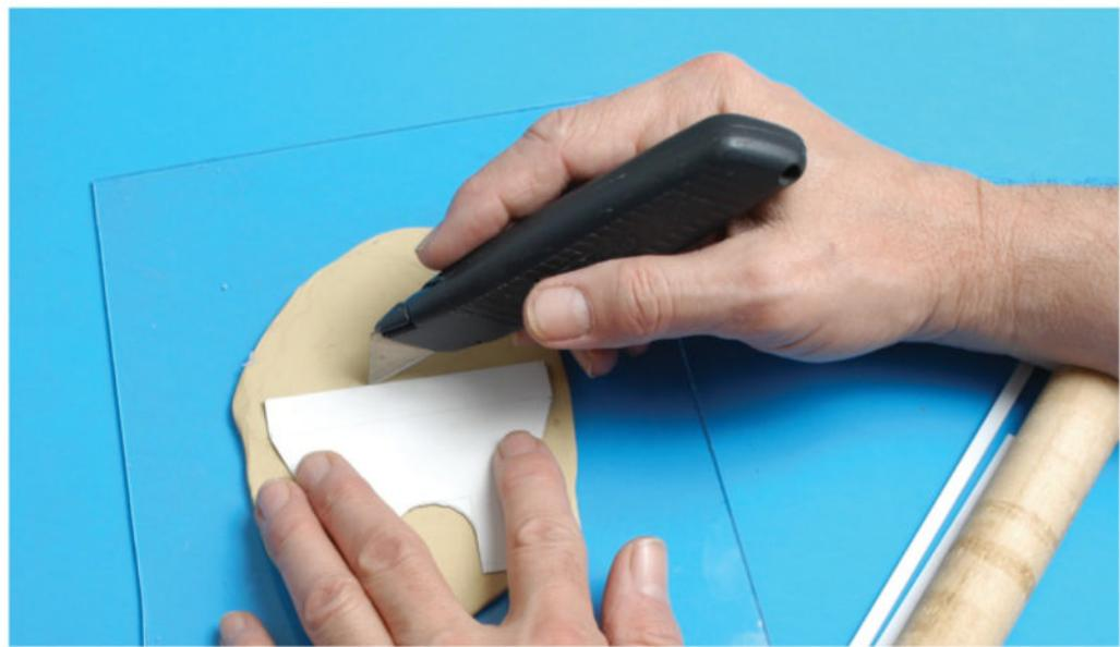
**2 From cardboard to clay.** With the clay rolled out, Howard set a cardboard template for the spandrel wall on top. Then he used a utility knife to cut the clay blank to shape.
