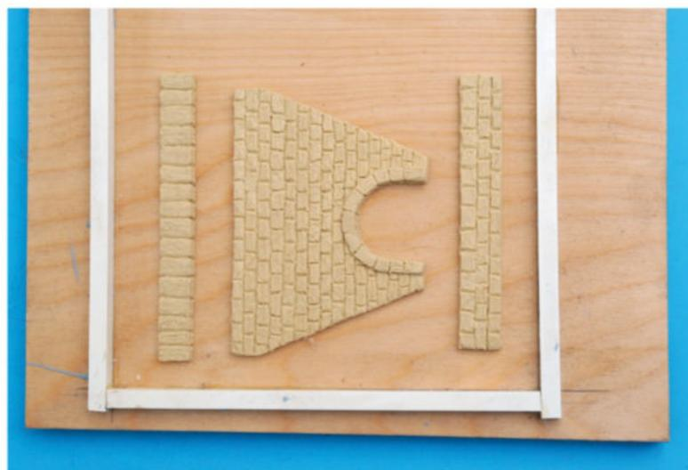
**6 Building the box.** With the clay masters finished, Howard placed the (left to right) capstones, spandrel wall, and parapet on a piece of wood. The styrene strips formed a wall to contain the silicone rubber used for the mold.
