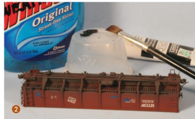
After removing the trucks and couplers, I brush-painted the new details to match the rest of the car. The color doesn't have to be a perfect match as the weathering will even things up. While I was at it, I brush-painted the air hoses flat black and the glad hands a rust color.
