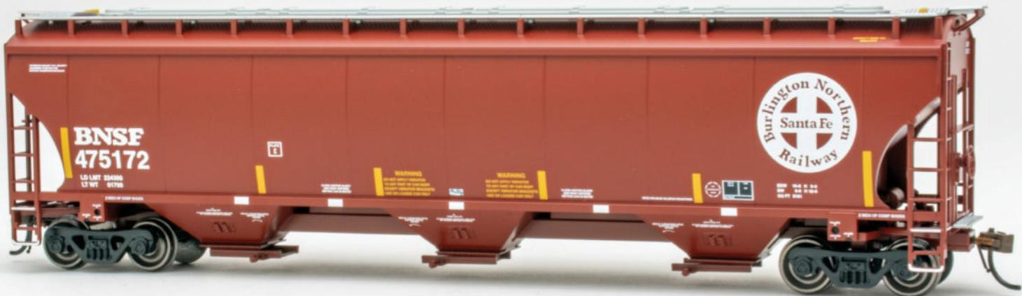
**A Trinity Industries** 5,161-cubic-foot capacity three-bay covered hopper is now part of Bachmann's growing lineup of modern HO scale freight cars. The injection-molded plastic model features screw-mounted roller-bearing trucks, metal wheelsets, and body-mounted E-Z Mate Mark II couplers.
