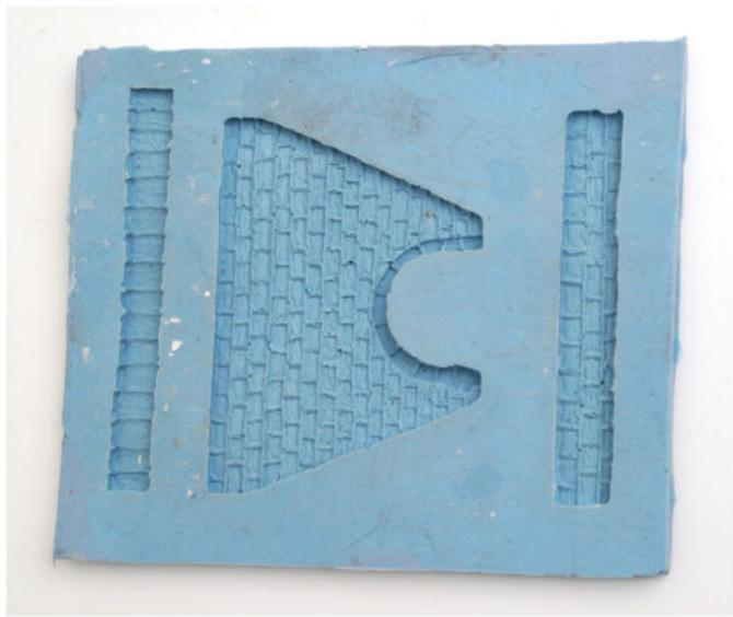
**7 Ready to use.** Here's what the finished one-piece mold looks like. Howard used Smooth-On OOMOO 30 silicone mold rubber for this project. The product is designed for basic molds like this.
