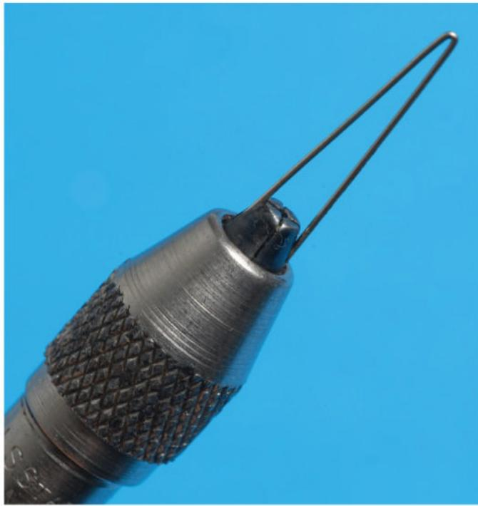
**3 Homemade solution.** A pin vise and a short length of nickel silver wire were all Howard needed to make a carving tool. The wire is a cutoff from the overhead for the trolley.
