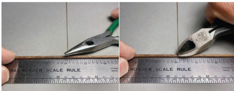
7 Jim pressed .020" brass rod into scribed and stained .100" square basswood to represent small bolts (left). He cut the rod as close to the wood as possible to finish each bolt (right). Jim inserted the bolts 9" on either side of 10 scale foot increments where timbers will be cut from the strip. He also inserted a bolt at the 5 scale foot center of each timber.
