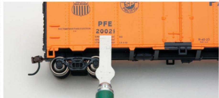
Alex Schneider recommends using a chisel blade in a hobby knife, bevel side down, to help remove factory-applied lettering. Cody Grivno photo
