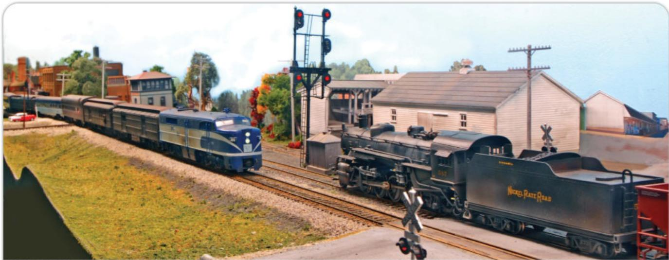
The signals governing the Nickel Plate Road (NKP) crossing of the Peoria & Eastern and the west end of the passing track at Veedersburg, Ind., on Tony Koester's HO railroad can inform the train crews of a variety of track conditions based on the three-color head atop the mainline signal and the two-color center head on the siding signal. Tony Koester photo
