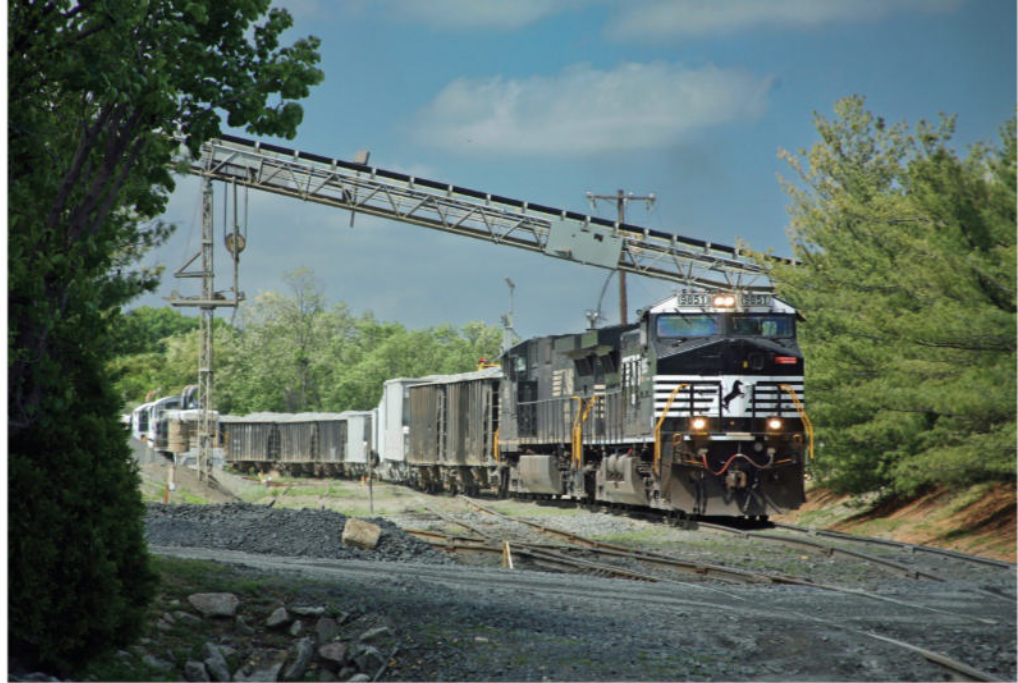
Norfolk Southern 9851, a General Electric Dash 9-40CW, is deep in the Vulcan Facility at Shirley Industrial Park. This photo illustrates how NS uses the heaviest engines to switch this branch.
