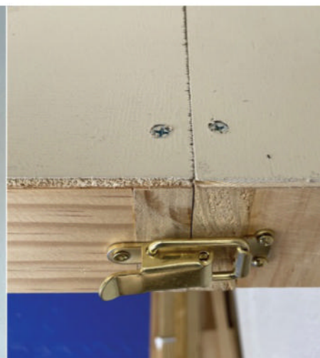
The layout in the stowed position is a snug fit around the cabinets. Note the Digitrax DCC system on a shelf under the benchwork. Latches at each end lock the folding part in the down position and pull the ends tight to maintain track alignment.
