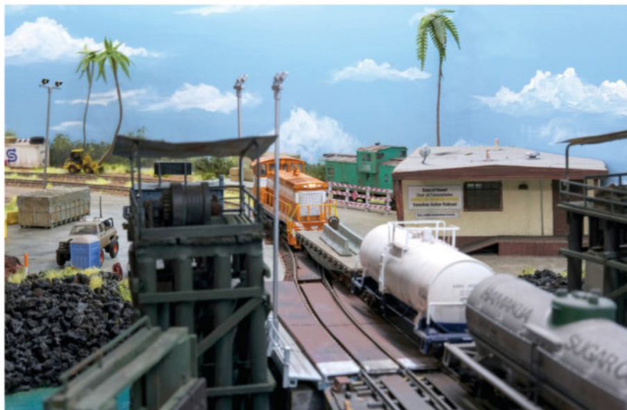
5 Kawaihae Harbor's SW1500 No. 50 pulls the morning inbound rail-barge cars using an old flatcar as a "reacher" car to keep the heavy locomotive off the barge slip. The flatcar is weighted down with a pair of Jersey barriers as ballast to improve tracking during heavy pulls off the barge.
