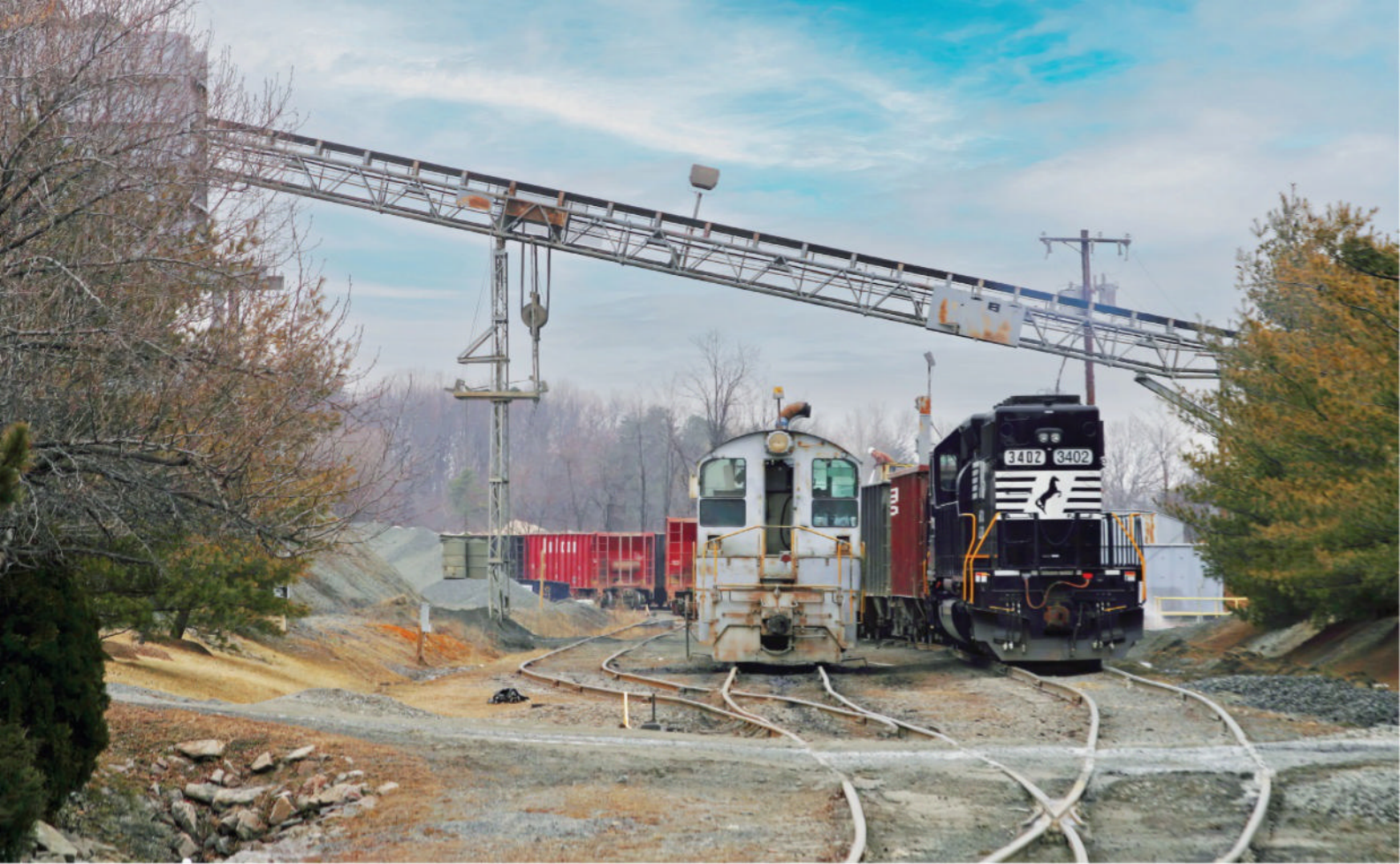
Norfolk Southern 3402, an Electro-Motive Division SD40-2, works cars at Vulcan Materials in the Shirley Industrial District. Vulcan's veteran end-cab switcher waits for its turn to work the hoppers.
