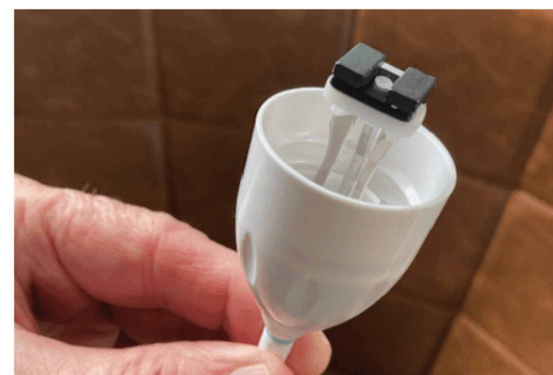
Paul Rising's Step by Step article "Rare earth uncoupling" appeared in the August 2025 issue. This image shows where the magnets are located on the toothbrush. Paul Rising photo
