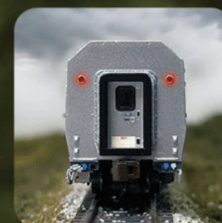
Working user-controlled LED marker lights on each end of the car
