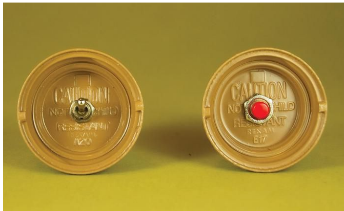
② The bottle caps can be fitted with either toggle or push-button switches. Jim painted his before installing them.
