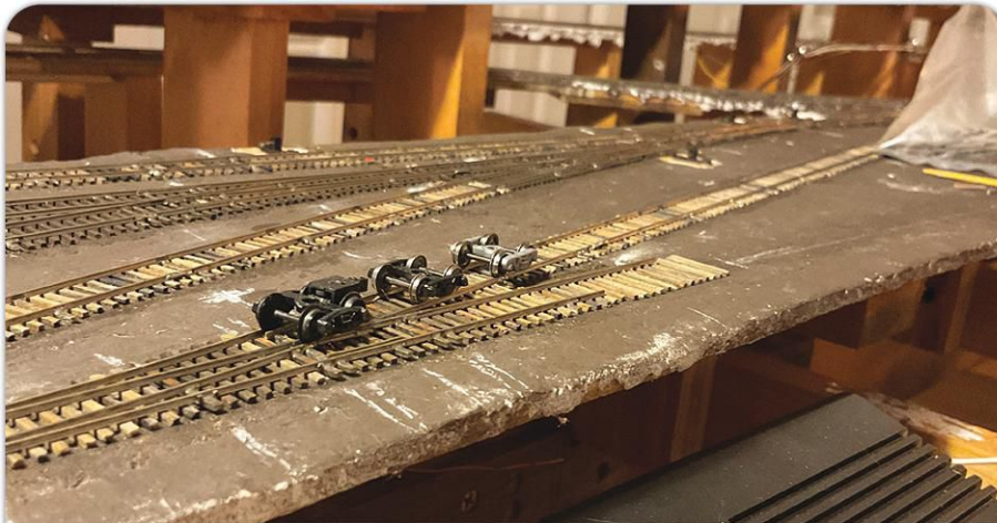
Richard Reitz is a proponent of smaller rail sizes in N scale, using code 40 rail with good results even with wheels that have larger flanges. Richard Reitz photo
