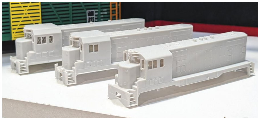
Atlas Model Railroad Co. displayed 3-D printed samples of its HO scale CF7 diesel locomotive at the Amherst Railway Society Railroad Hobby Show in late January. The Master Line model will be offered with round and angled cabs. Bryson Sleppy photo
