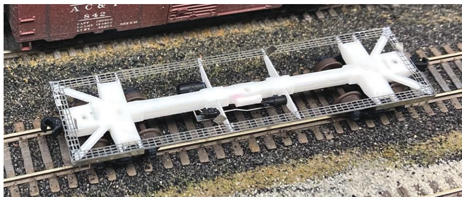
7 See-through platforms. Inspired by etched-metal boxcar running boards from Plano, Steve made see-through tank walkways for his models. The hazmat placards on the sides and ends, part of each etching, were folded up at a right angle.
