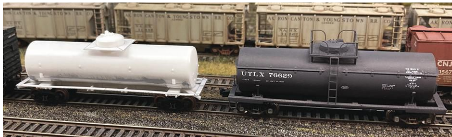
4 Test time. Steve turned to etched-metal parts for the walkways and dome platforms. He printed the artwork and placed it on the model to make sure everything would fit before sending the files off for production.
