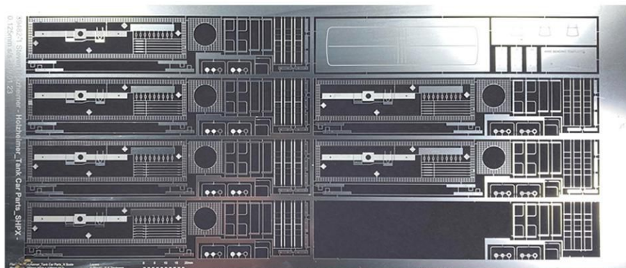
4 Test time. Steve turned to etched-metal parts for the walkways and dome platforms. He printed the artwork and placed it on the model to make sure everything would fit before sending the files off for production.
