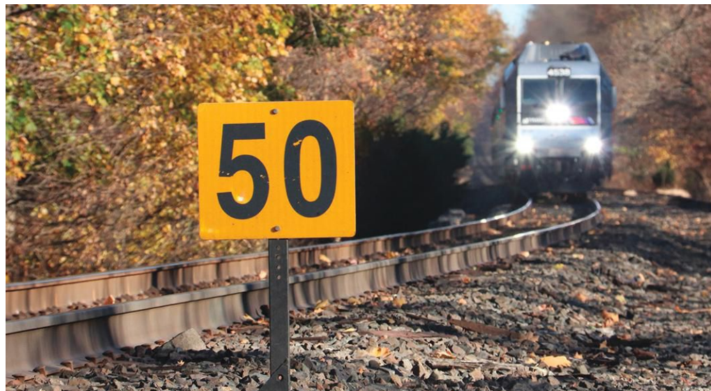
This temporary advance speed sign in Lebanon, N.J., frames a westbound New Jersey Transit train approaching in the background on Nov. 15, 2024. The sign warns eastbound engineers to begin braking for a 50 mph slow over track under repair. Jerry Dzedzic photo
