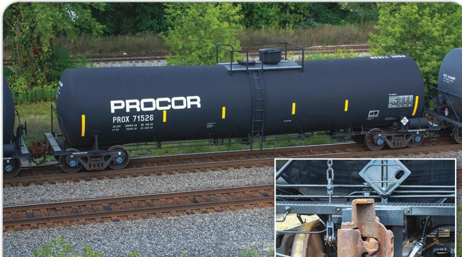
Contemporary tank cars, such as Procor Limited No. 71526, are fitted with double-shelf couplers to prevent vertical separation in the event of a derailment. The inset photo shows a Wabtec SE60EE double-shelf coupler. Cody Grivno photos
