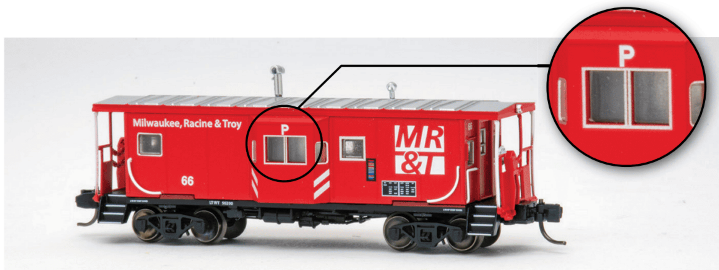
Milwaukee, Racine & Troy N scale bay-window caboose No. 66, produced by Bluford Shops, features the letter "P" on both sides. This indicates it's a pool caboose that can be used throughout the MR&T system. Cody Grivno photo
