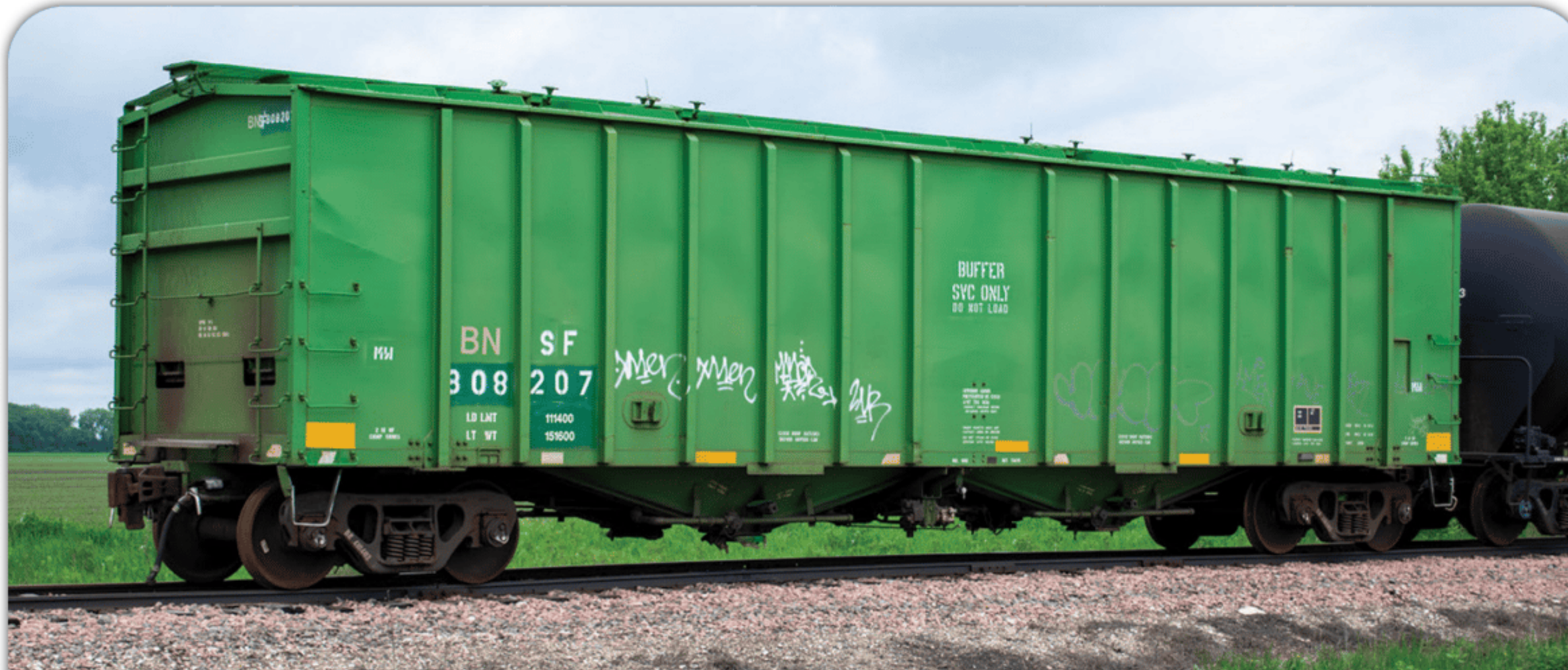
BNSF Ry. 808207, a General American 4,180-cubic-foot capacity Airslide covered hopper, is an example of a car assigned to buffer service. The stencil on the wide body panel reads BUFFER SVC ONLY DO NOT LOAD. Cody Grivno photo
