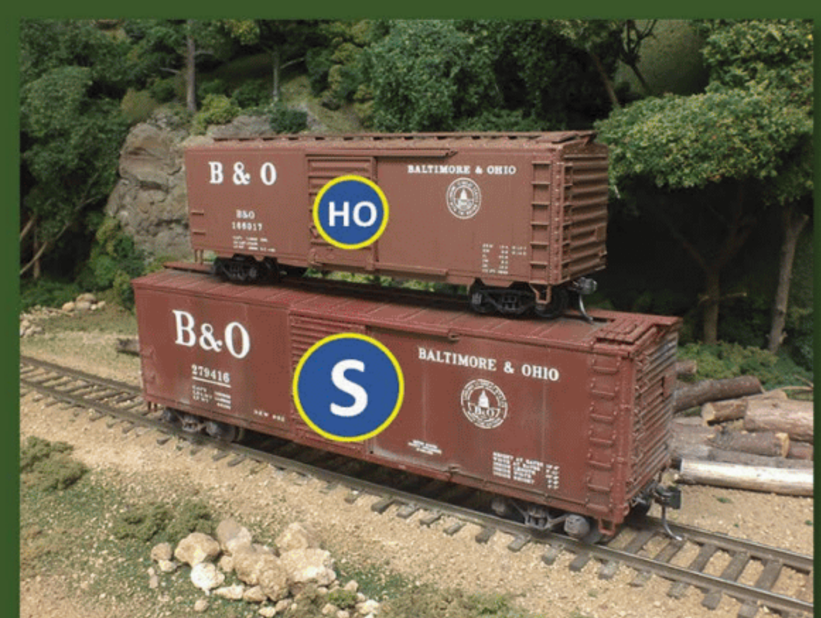
S scale is just 36% greater in linear dimension than HO but has a volume 250% larger.
