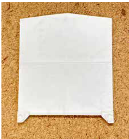
1 End game. Paul made a pattern for the car ends from .040" plain styrene sheet. He added a .010" styrene overlay with embossed rivet detail applied with a NorthWest Short Line die.
