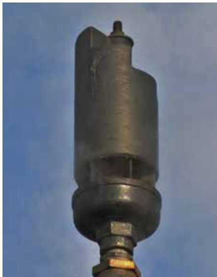
Sunrise gleams on the whistle of Black River & Western No. 60, a former Great Western 2-8-0 built by Alco in 1937. Though the now familiar grade crossing whistle signal of long-long-short-long was written into the Standard Code in 1928, not all railroads adopted it right away. Jerry Dziedzic photo
