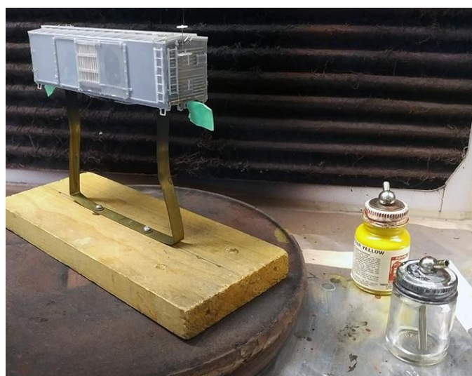
2 A simple solution. David used punched steel strapping, a wood block, and screws to make this painting jig for his resin freight cars. The green masking tape is covering the couplers.
