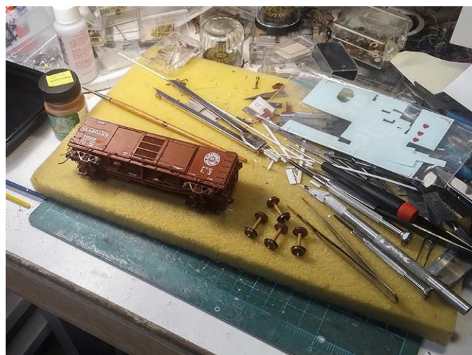
3 At the bench. Though David's workbench looks busy, there's a method to it. The water, setting solution, and brushes are at left. Unused decals are stowed in a plastic bag toward the back. The tweezers and dividers are used for applying and aligning the lettering.
