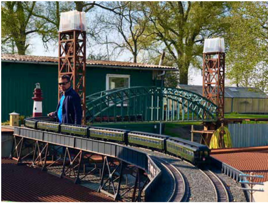
4 Oliver checks a turnout on the wye near the loop at the shop end of the layout. The lift bridge in the background works; the chain drive in the towers can lift it to give more than 7 feet of clearance for people and construction equipment.
