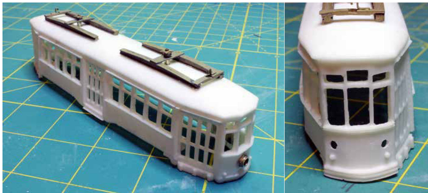
③ Time for lights. To make the holes for the headlight and taillights, Harvey started with a smaller bit and filed the size of the opening for a tight fit. The headlight casting came with the shell.
