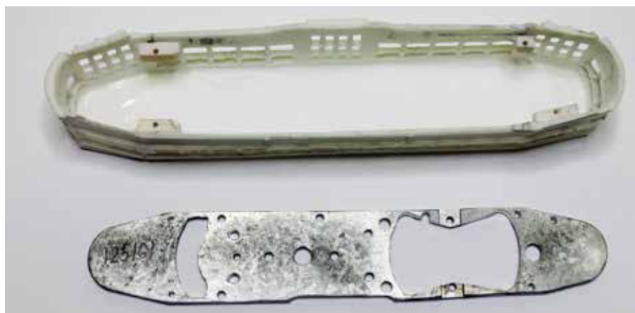
② Making modifications. Here are the changes that Harvey made to the floor. Note the holes drilled in the floor that mate with the four small chunks of resin that were glued to the shell.
