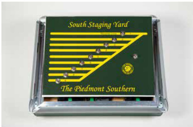
5 The snap frame from SECO can be opened for easy access to the control panel, allowing it to be lifted out. Larry screwed the frame on top of a wooden enclosure.
