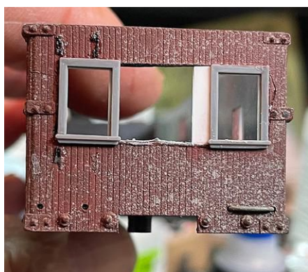
After using a nibbler tool to remove the material in the window opening, Jim tested the fit of the Tichy Train Group windows and the styrene spacers.
