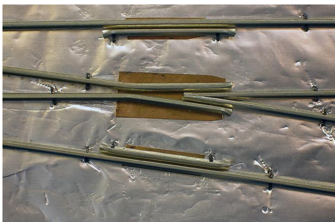
7 Guardrails are formed and spiked down on top of a .005" brass shim. The flangeways are carefully checked to be in compliance with an NMRA clearance gauge.
