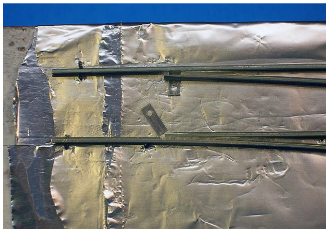
6 Metal tabs are soldered under the point rails to connect them to the turnout switch rod. They extend under the stock rails to prevent them from riding up and out of their position.
