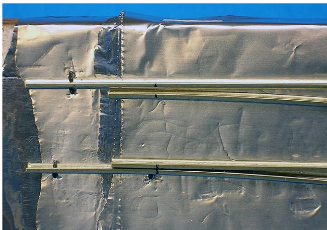
5 The point rails are marked where they'll terminate, and the stock rails are marked where they'll be notched so the points will seat properly.
