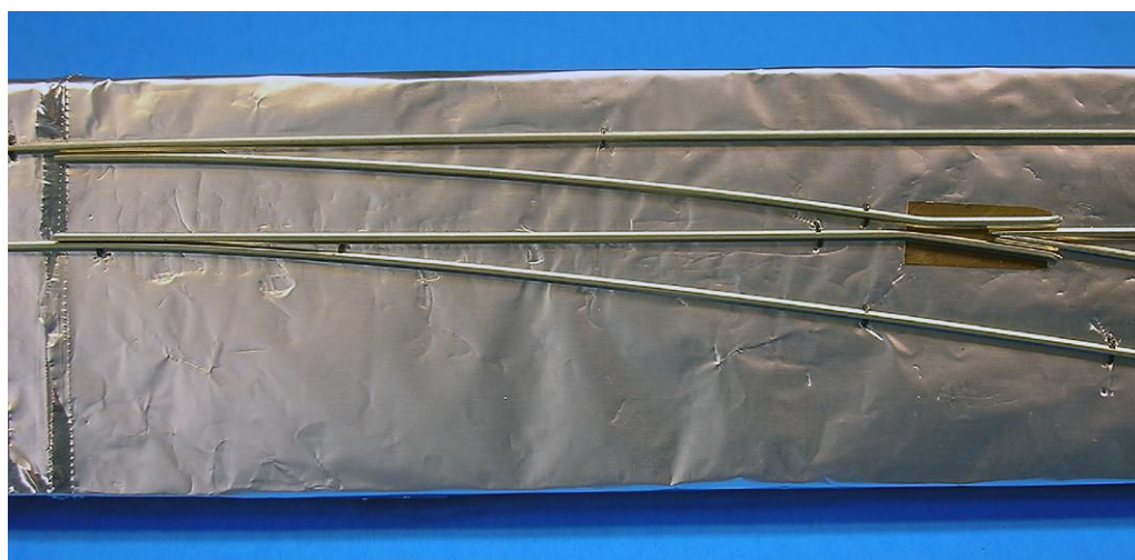
4 The points and closure rails are single pieces without hinges.
