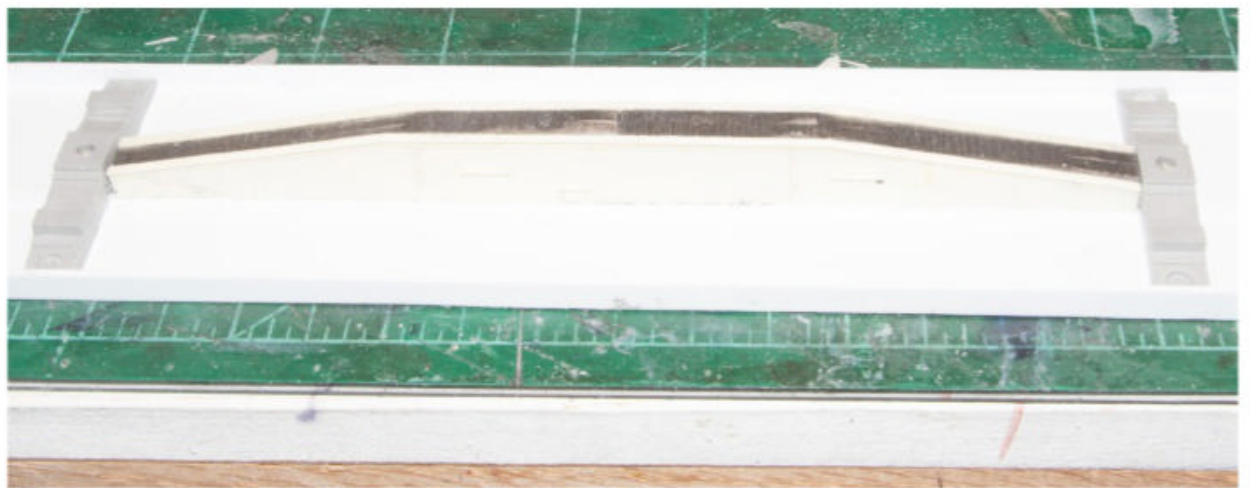
4 Attaching the sills. Weights from Scale City Designs are concealed between the cast-resin center sills. Charles attached the resin sills to the metal weights with cyanoacrylate adhesive.
