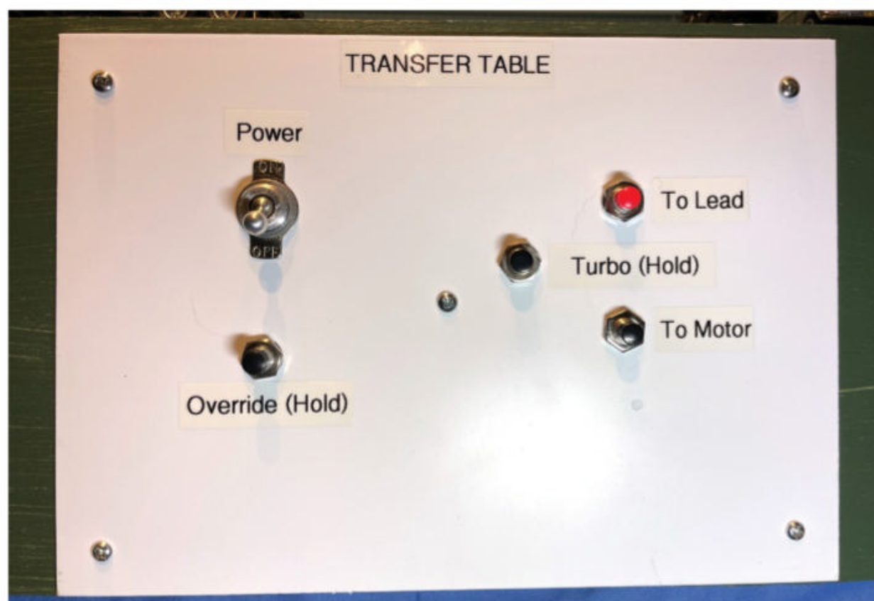
6 The control panel gives operators several options when controlling the transfer table. The “turbo” option moves the table at double normal speed when the button is held down.
