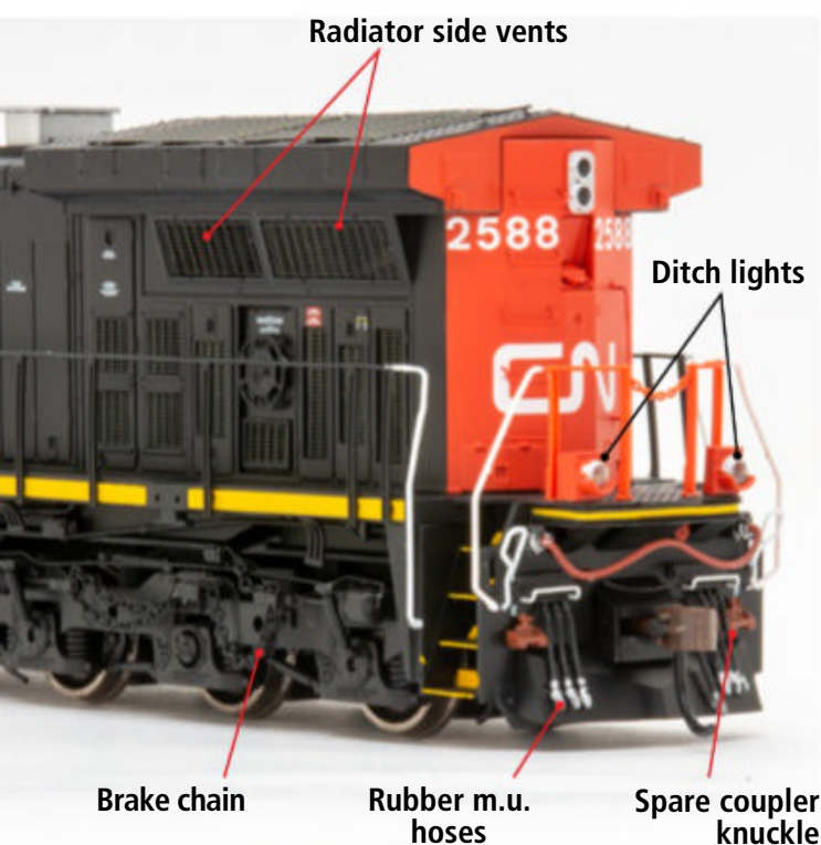
The rear of the CN 2588 is loaded with details. The etched-metal body and radiator side vents are see-through.
