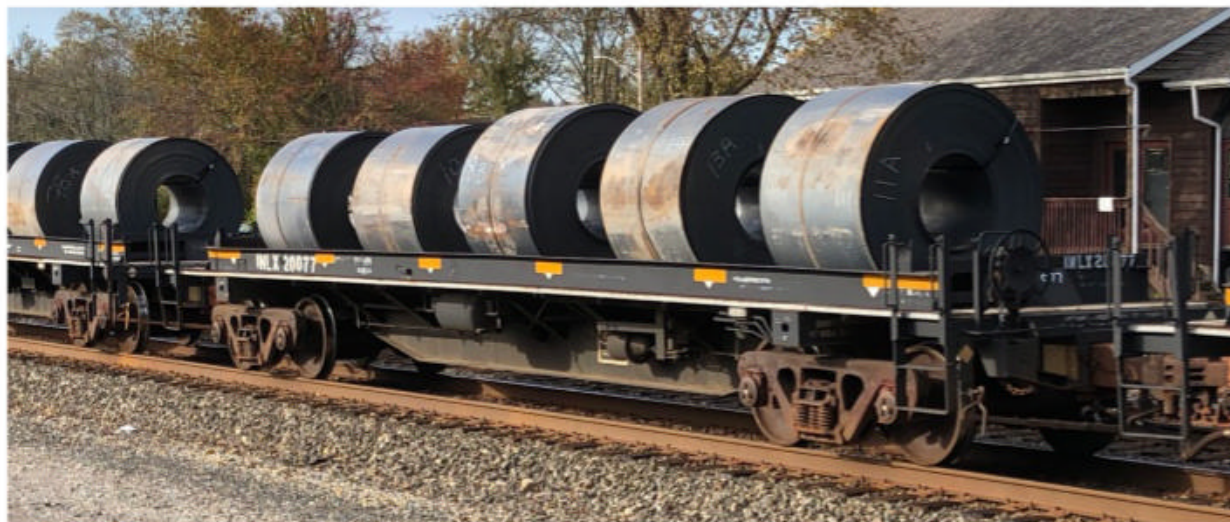
A coil steel car moves through Chesterton, Ind., in an eastbound Norfolk Southern train on Nov. 7, 2021. Car weight capacity governs how steel is moved on the railroads. Thomas E. Hoffman photo
