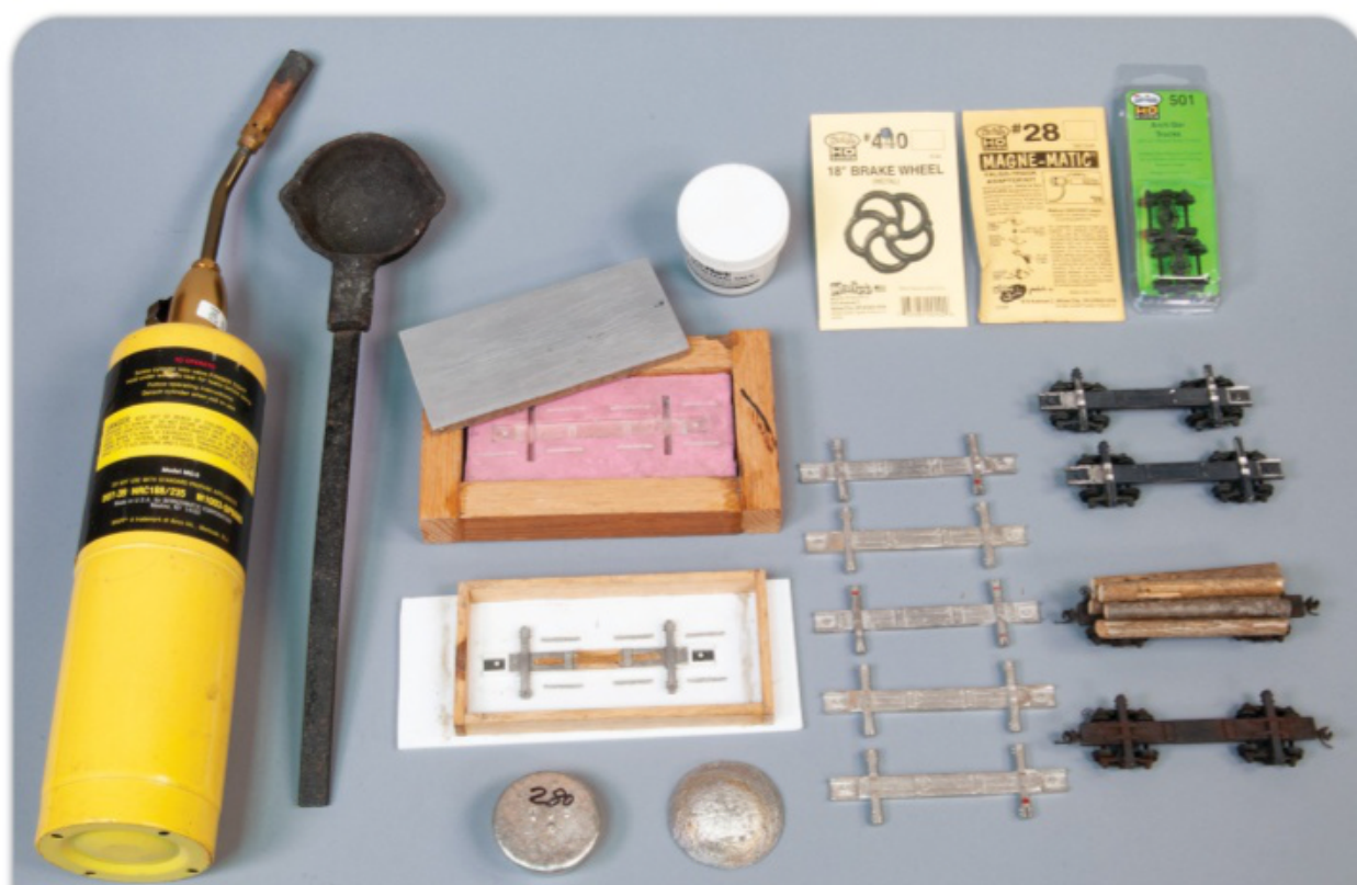
The materials used in casting and finishing a metal log car are shown. From left to right are a propane torch and metal ladle, the silicone mold, the master, detail parts, cast frames, and cars in various stages of completion.
