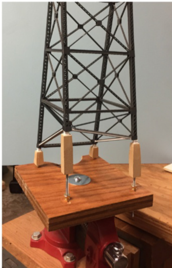
11 The full tower and support assembly is shown attached to its horizontal support.
