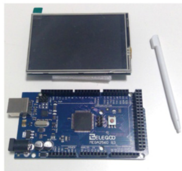
3 A winning combination. Colin paired up an Arduino microcontroller (bottom) with a liquid-crystal display touchscreen. A stylus is shown to the right.
