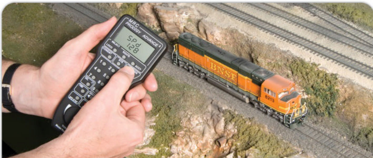
An operator programs a locomotive using a Digital Command Control throttle. Here's what to do when a DCC locomotive won't hold an address. Model Railroader staff photo
