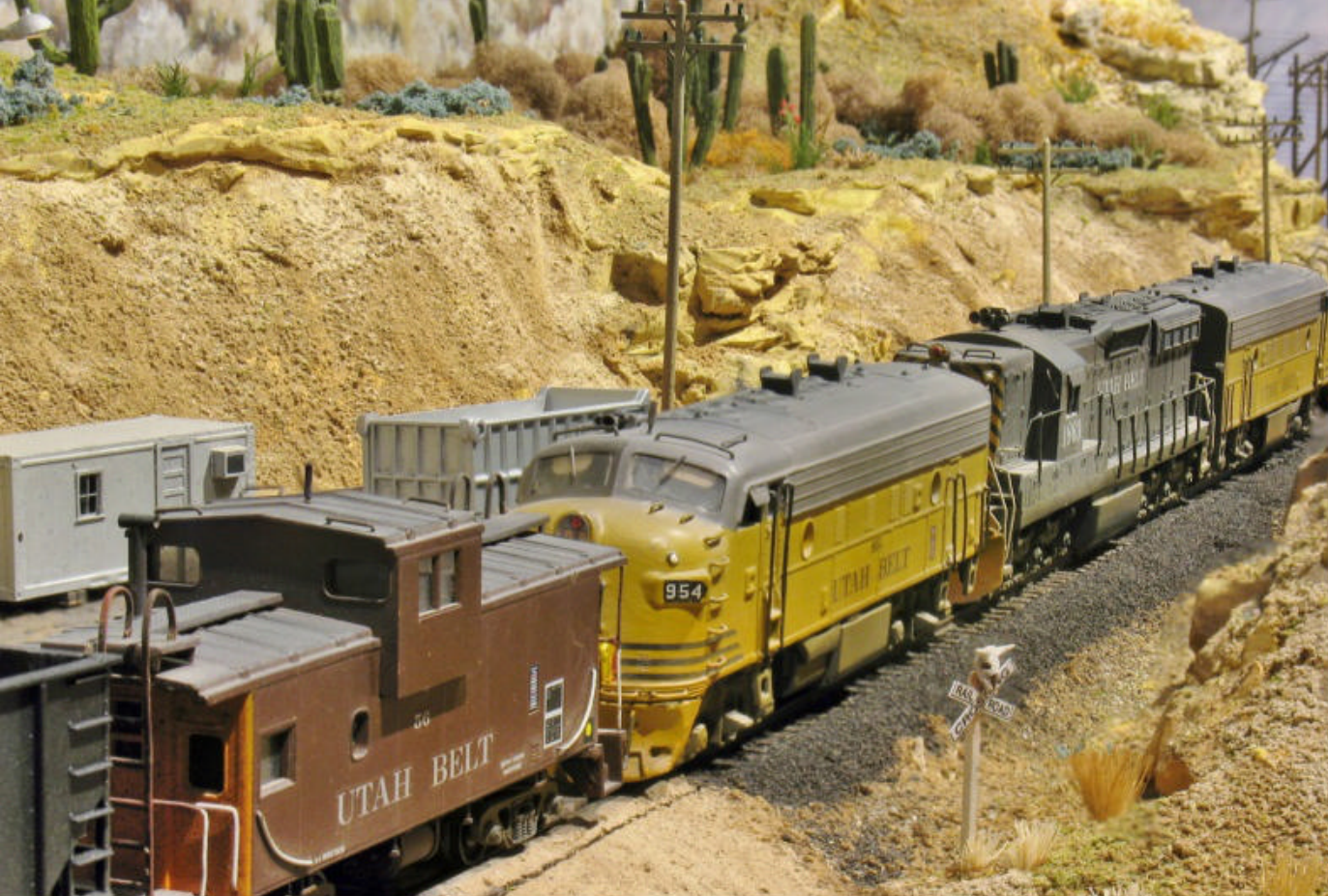
③ The way it used to be. This circa 1980 image shows a pair of Electro-Motive Division F7As and an SD9 helping a westbound train at Coal Bank. These former mainline units were serving out their final years on the Utah Belt in helper service.
