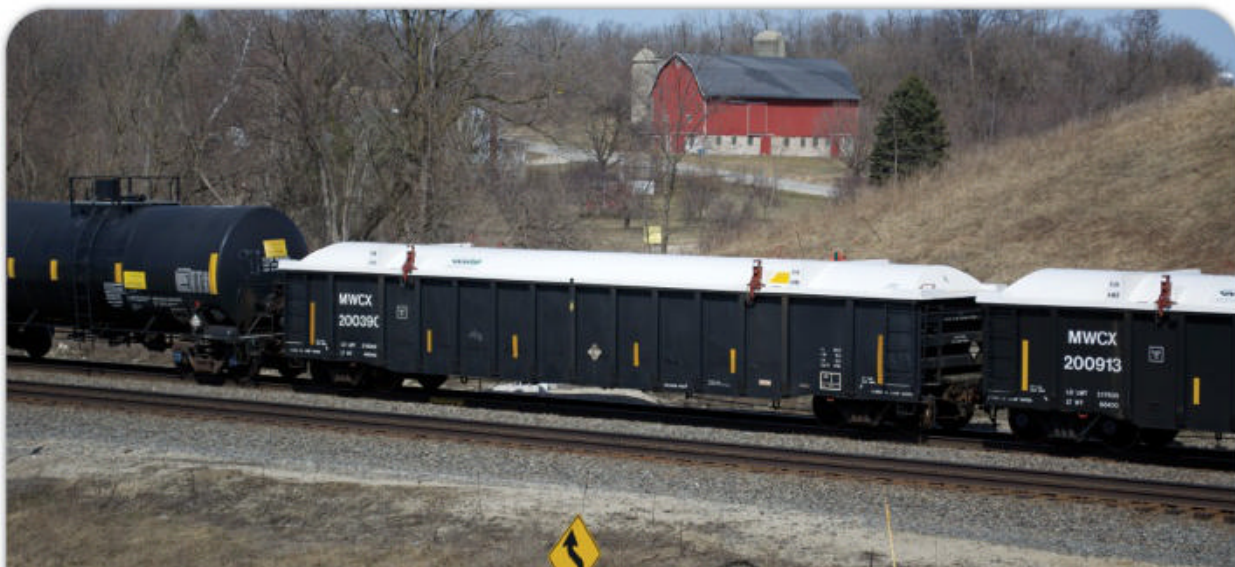
Midwest Railcar Corp. no. 200390, a 2,791-cubic-foot-capacity gondola, rolls through Ackerville, Wis., in a Canadian National freight train on March 21, 2021. The 52'-6" car is fitted with a Fiberglass cover produced by Ecofab. Cody Grivno photo
