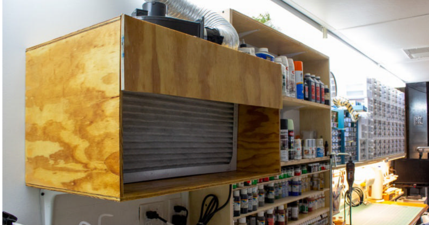
A custom-built spray booth with a standard furnace filter and powerful fan was added to replace Richard's antiquated one. Shelves to the right keep paint handy.
