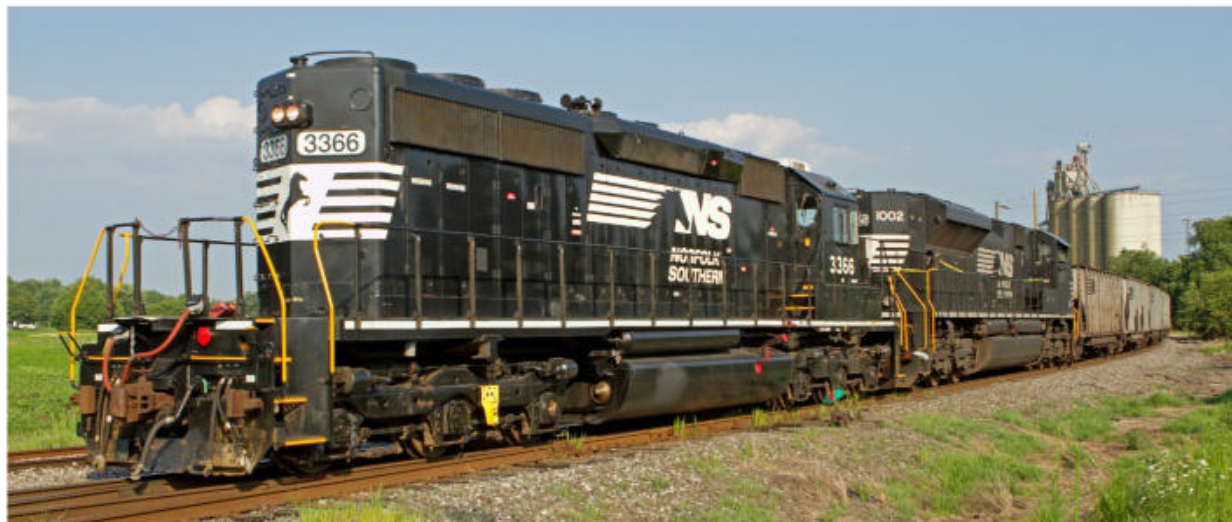
Norfolk Southern no. 3366, an Electro-Motive Division SD40-2, leads a train of empty coal hoppers in Harrington, Del., in July 2011. The bulging section on top of the long hood, above the herald, is the dynamic brake enclosure. Jason Walter photo
