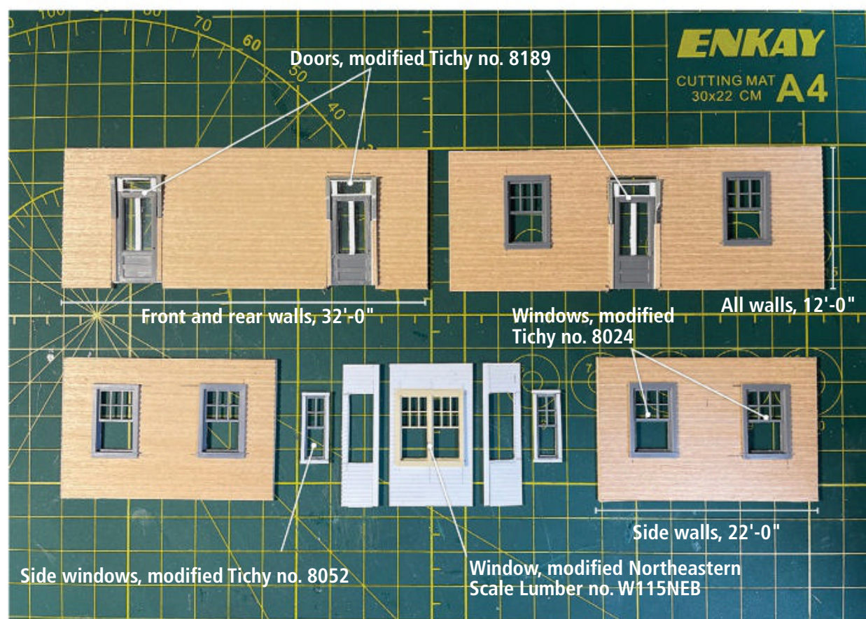
2 Bits and pieces. Tom cut out the walls and openings for the doors and windows prior to assembly. He built the operator's booth out of styrene.
