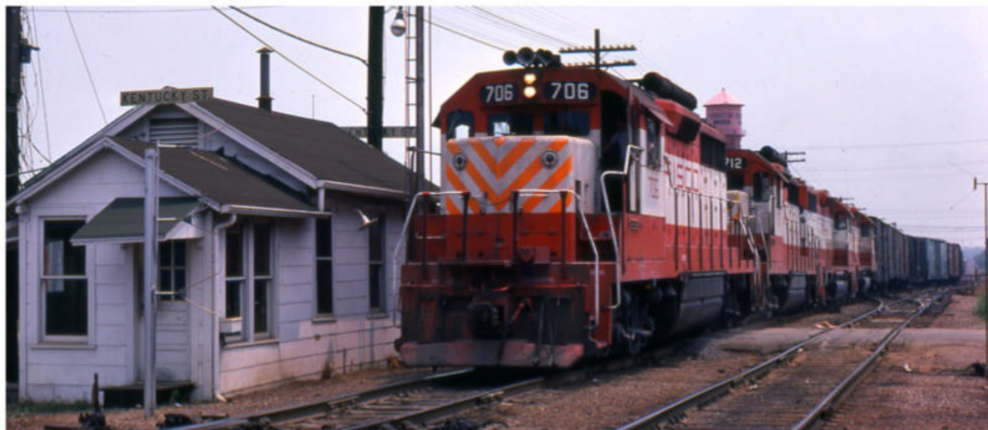
A sultry July 3, 1975, finds Frisco no. 706, an Electro-Motive Division GP35, leading a westbound past Kentucky Street Tower. Frisco GP35’s carried their air reservoirs on top of the long hood because the extra-large 3,000-gallon fuel tanks the railroad specified left not enough room under the frame. Jerry Dziedzic photo
