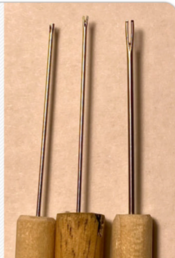
David Varholy cut off the ends of the eyes of three sewing needles and inserted them into dowels to make precision applicators. David Varholy photo
