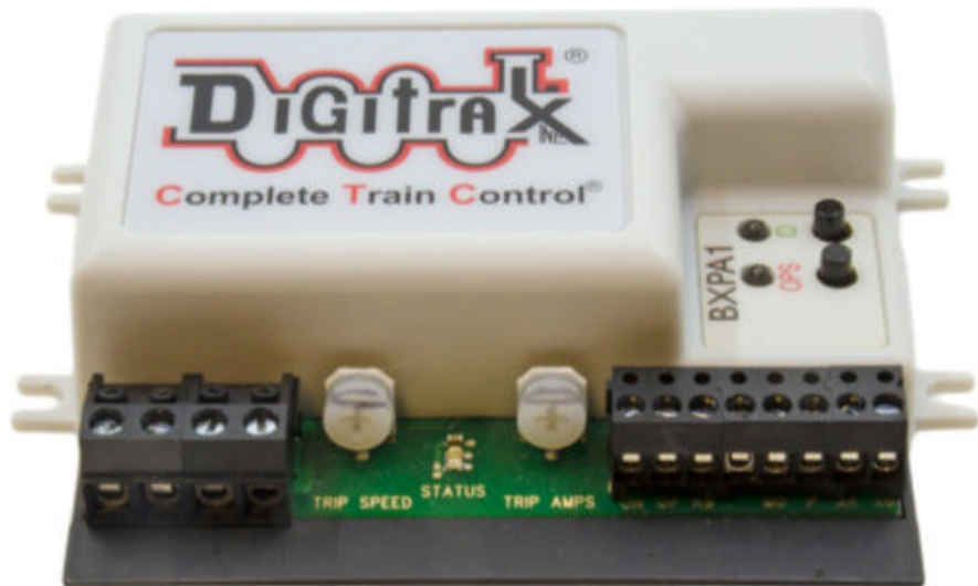
3 Digitrax BXPA1 auto-reversing unit and block detector.
