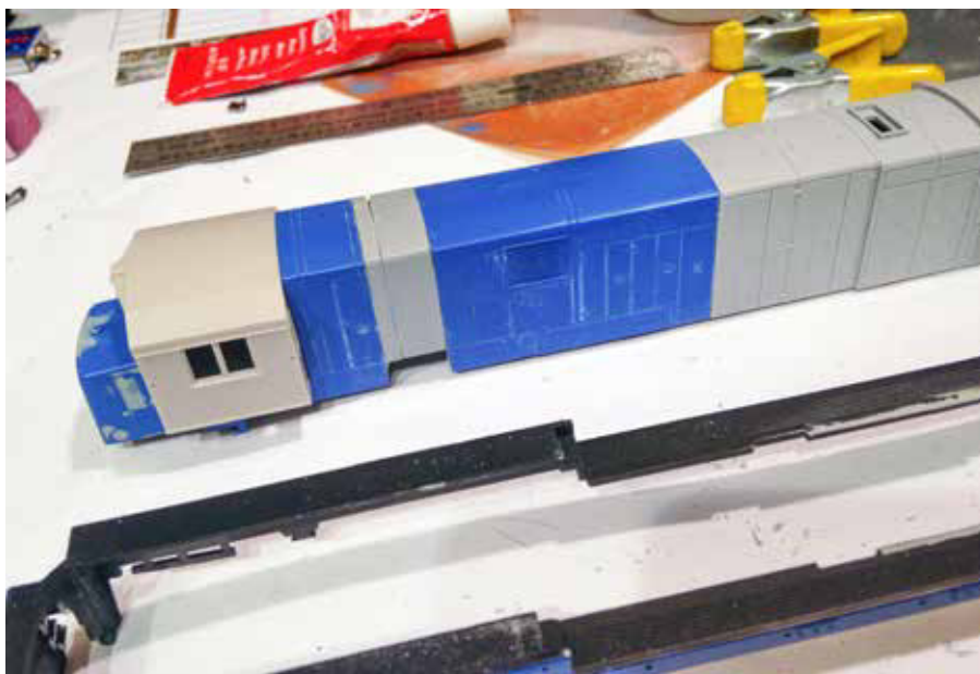
3 Critical test. It is critical in a major kitbash to test-fit components. Here, the unaltered Atlas C30-7 frame is used to test the assembly of other components.
