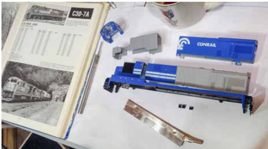
1 The first cuts are the hardest! Using reference book photos, Dave cut the C30-7 shell (in blue) and the B23-7 shell (gray) to begin creating the long hood.
