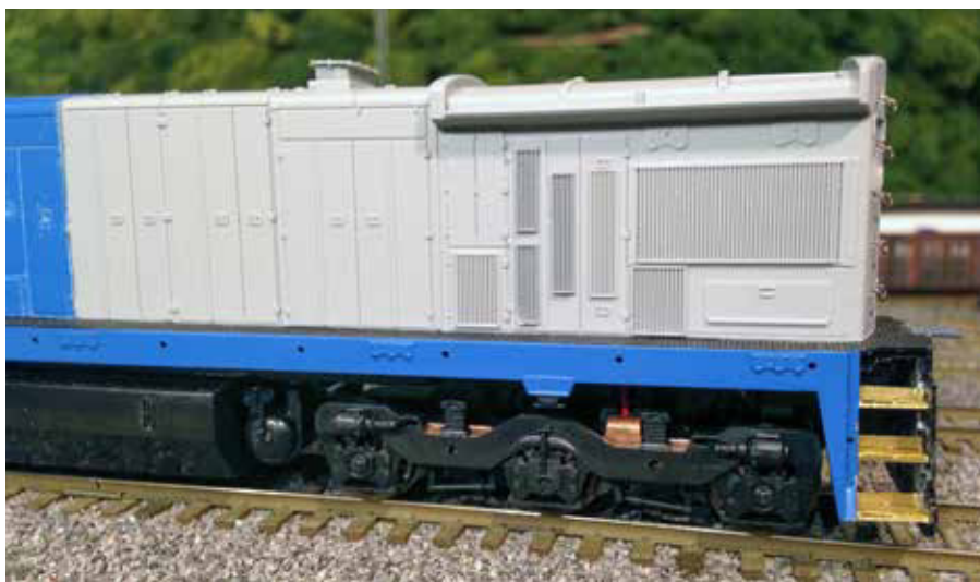
2 Bringing up the rear. The B23-7 shell provides the entire rear of the long hood, with the addition of extra intakes from Hi-Tech Details.
