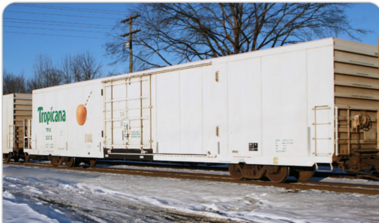
A Tropicana refrigerator car is seen on the Juice Train northbound on the CSX RF&P subdivision, passing through Doswell, Va., in February 2010. Reefers like this are used for cargos that must be kept cold; insulated boxcars are for shelf-stable but temperature-sensitive freight. Alex Mayes photo
