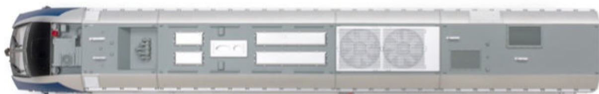
The five-chime horn and an array of radio antennas are added details on the roof. Radiator fan detail is molded in place and painted, creating a convincing effect.
