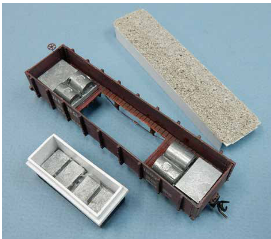
3 Adding weight. Assorted Woodland Scenics weights designed for Pinewood Derby cars brought the gondola up to 2\frac{3}{4} ounces. The removable load conceals the weights and interior modifications.
