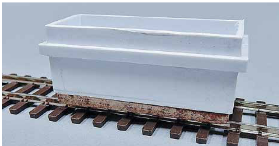
1 Basic box. John used styrene strip and sheet to build the cleaning box. He used 5-minute epoxy to attach \frac{1}{8} "-thick tempered hardboard to the bottom of the box.
