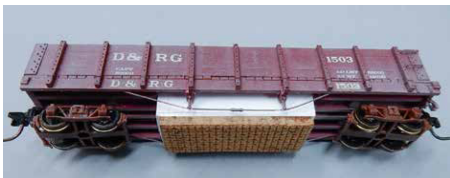
2 Easy installation. John cut a hole in the bottom of this HOn3 gondola to accept the cleaning box. The box should slide and move freely in the opening.
