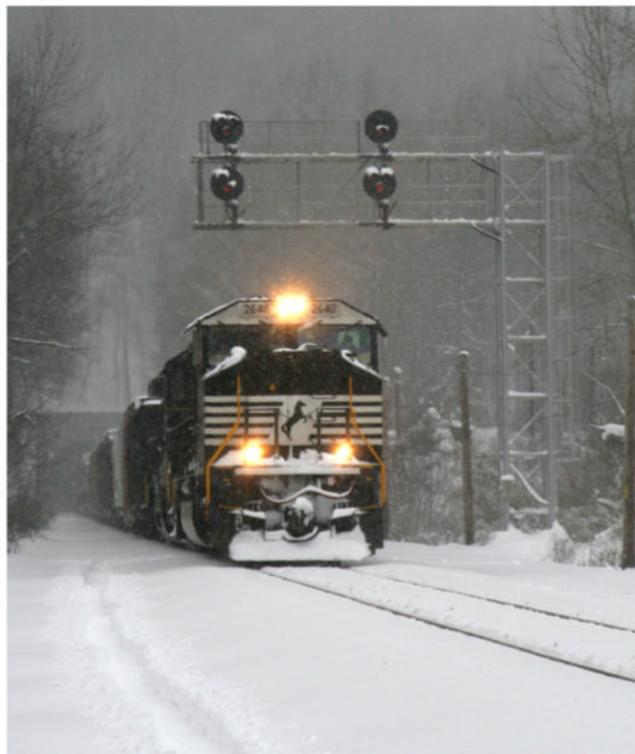
Centralized Traffic Control signals guard CP64 at Musconetcong Tunnel on Norfolk Southern's Lehigh Line, past which SD70M 2640 and a C40-9 muscle eastbound manifest 32A through a blizzard on Feb. 12, 2006. Jerry Dziedzic photo
