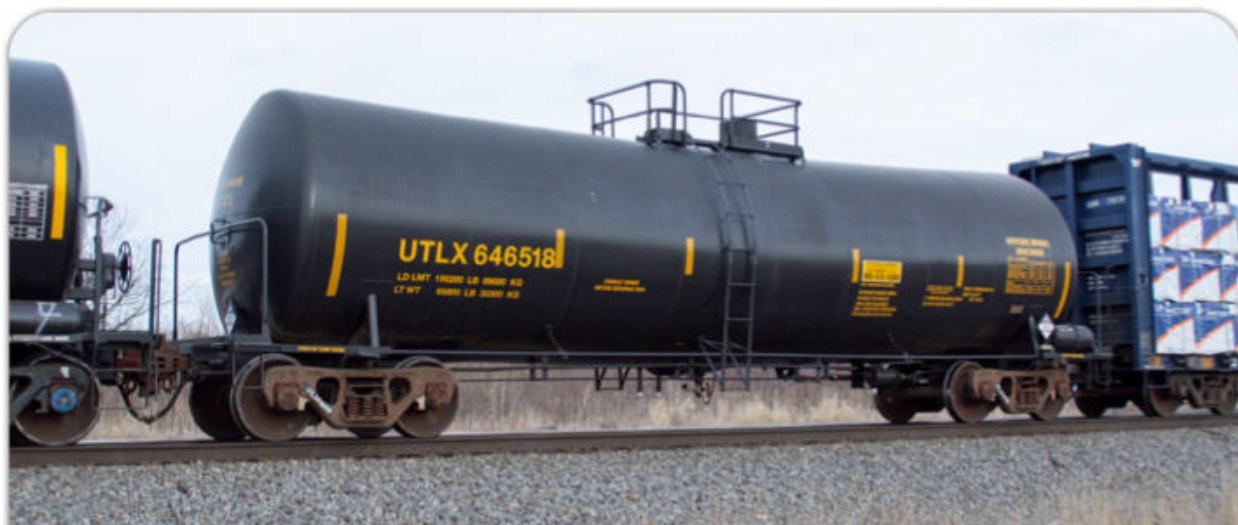
Union Tank Car no. 646518, a 20,500-gallon Funnel Flow tank car, is part of a southbound Canadian National freight passing through Lisbon, Wis., on March 20, 2018. The car is transporting methylene diphenyl diisocyanate, a chemical used in making polyurethanes, such as flexible foam insulation. Cody Grivno photo
