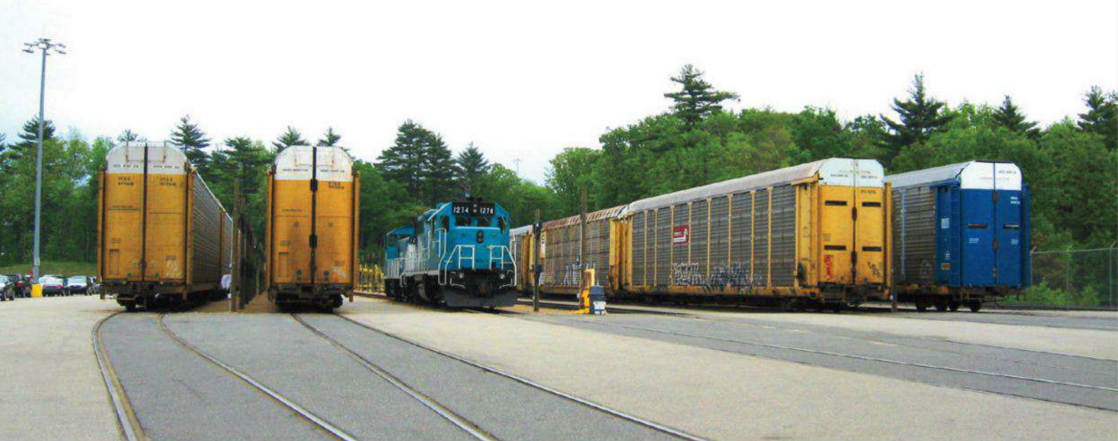
This view toward the unloading tracks at East Brookfield, Mass., shows the track layout, a light pole for night operations, and two leased (by the East Brookfield & Spencer RR) RTEX Electro-Motive Division locomotives.
