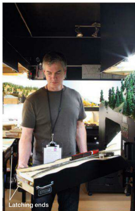
Mark built swing and lift gates to allow access while maximizing operations. Left: Train traffic into the mushroom is by way of a swing gate at South Slocan. The ball detents and hard wood runner visible on the gate lock into matching parts mounted on the benchwork. A bicycle neck bearing smooths the gate's pivoting motion. Right: A short lift gate facilitates entry into the mushroom. When down, it's a 4'-3" duckunder; raised, it's a 5'-1" nod-under.
