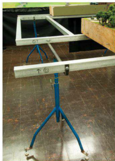
The railroad is supported on an aluminum frame, which is carefully leveled before the layout sections are slid into place. Fine adjustments are made at the foot of each tripod leg.
