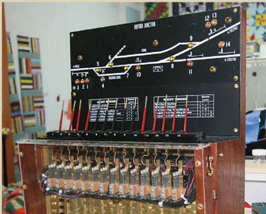
Don Ball, who's modeling a California shortline railroad set in 1895 ( Model Railroad Planning 2011 ), scratchbuilt this working interlocking machine to control the plant at Orford Junction. Don Ball photo
