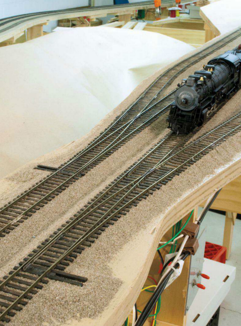
3. Andy enjoys building track from scratch and has handlaid all the track on his layout so far. Here are two Santa Fe-design no. 6½ turnouts at the lower (west) end of Cajon station. On the left is a standard turnout, and on the right a spring switch for the heading-out end of the westward passing siding.
