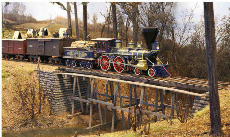
4. Handsome 4-4-0 McCallum , built by Mason, leads a train across the Clairborne Creek trestle. Brigadier General and military engineer Herman Haupt developed the W-bent design to expedite wartime construction.
