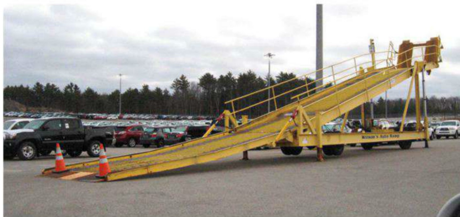
A Wilson's Auto Ramp can be used to unload from either end of all tracks. Once positioned, the ramp is raised on jacks for stability.
