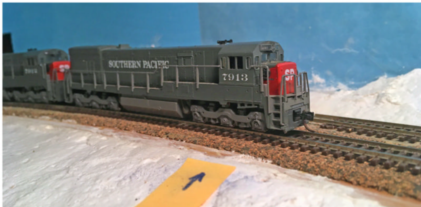
It's a bit hard to see, but the bad joint between plywood surfaces that was causing derailments is just above the point of the arrow. This is the after photo. Roen Kelly photo
