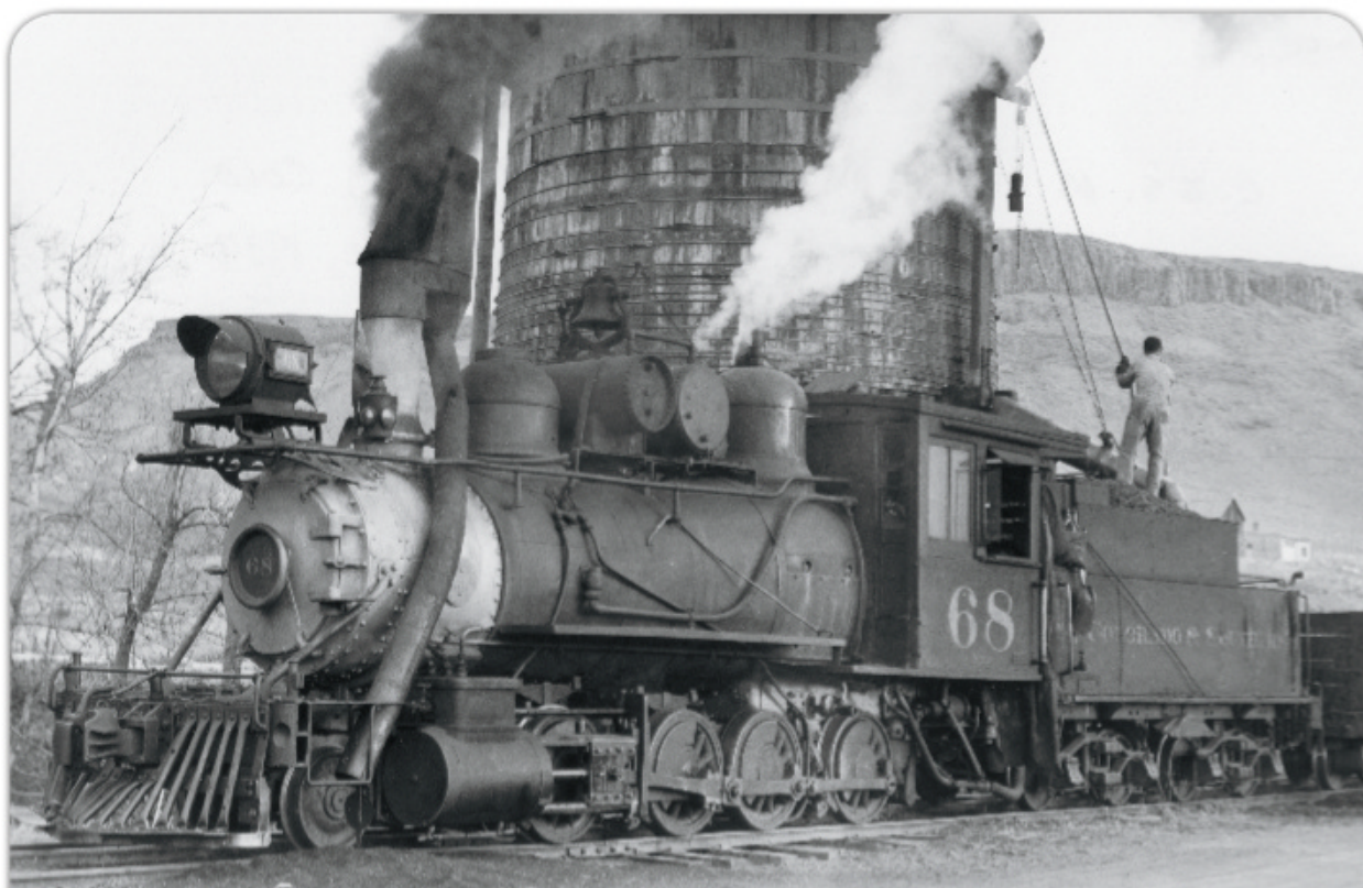
Colorado & Southern narrow-gauge 2-8-0 Consolidation no. 68 takes on water at Golden, Colo., on Jan. 30, 1939. As smoke escapes the front of the locomotive's "bear trap" stack, cinders are caught by the device and routed into the pipe on the side of the smokebox for later disposal. R.H. Kindig photo
