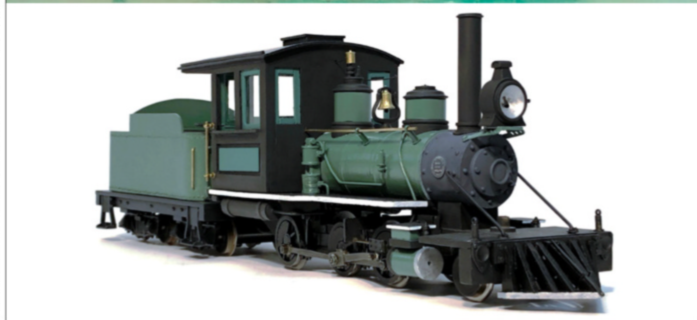
As you can see, this 1:20.3 (or so) narrow gauge Mogul was built primarily from wood – "an excellent material for such a purpose," according to builder Tom Piccirillo. Tom Piccirillo photos
